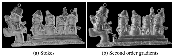
Figure 8: Comparison of estimated per pixel specular roughness with the technique of Ghosh et al. [2009]. (a) Specular roughness estimated from the Stokes measurements of constant full-on illumination. (b) Specular roughness from polarization difference imaging of second order spherical gradients.
