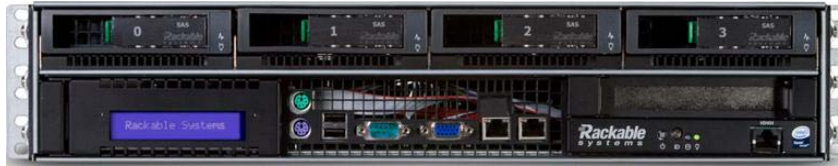
Figure 1-2 An SGI Rackable C2005 Server
