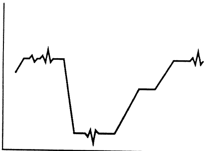
Figure 6: The analog input signal. Note the "noise" on the signal's peaks.
