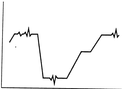
Figure 3: The analog input signal. Note the "noise" on the signal's peaks.
