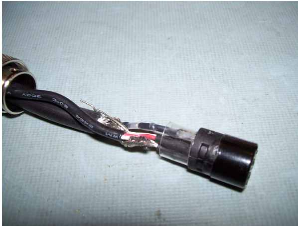
Replace the plastic ring and position shield and drain wire facing back
