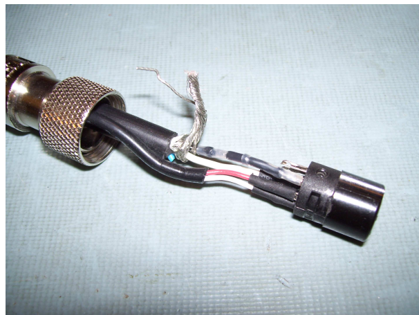
Re-solder the black wire to pin 7
