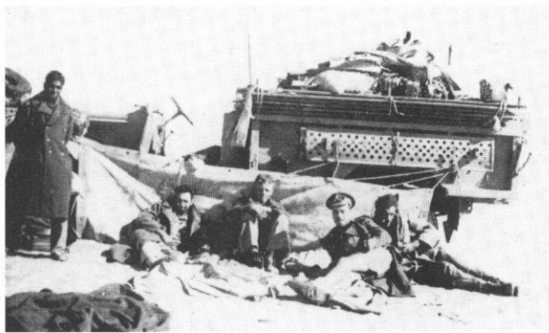
Patrols carried everything needed for operations and for comfort stowed in the back of their trucks in a logical order, like a ship at sea. This Chevrolet 1533X2 W/T truck of the Indian Long Range Sqdn. has its tarpaulin rigged as a comfortable 'bivvy' during a midday halt. The short 3-ft. whip aerial indicates that the signaller is trying to communicate with a base not too far distant.
