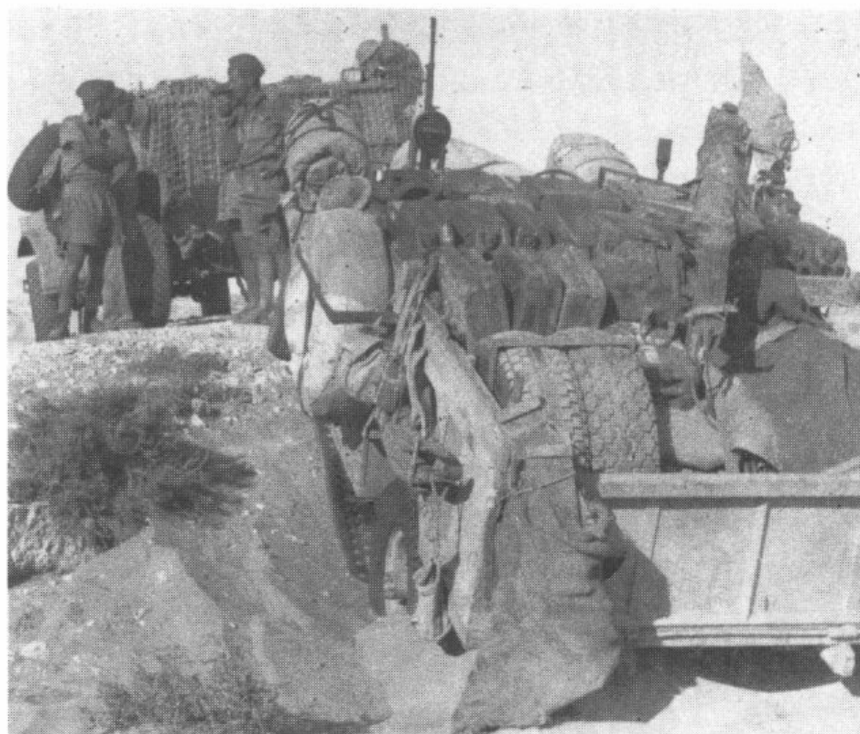
Sand channels, devised by Bagnold, were vital equipment, and patrols soon became highly proficient at 'unsticking' vehicles in a hurry—for lack of mobility meant death if caught in the open by enemy aircraft. Here an F30 is towing a 1533X2 up sand channels; as usual, the bulk of the load is petrol, closely followed by spare tyres. Note Vickers medium machine gun on central pillar mount, shrouded in canvas, and additional Vickers KOs each side of the cab.
