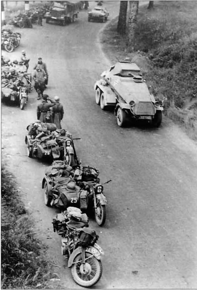
German solo and combination motorcycles of a reconnaissance battalion line a road during a brief halt in Russia, summer 1941; the white 'G' painted on the headlight covers identifies Panzergruppe Guderian. The heavy armoured car is an SdKfz 231 Waffenzugwagen (weapons car) armed with a 2cm cannon and 7.92mm machine gun. (Courtesy Concord Publications)
