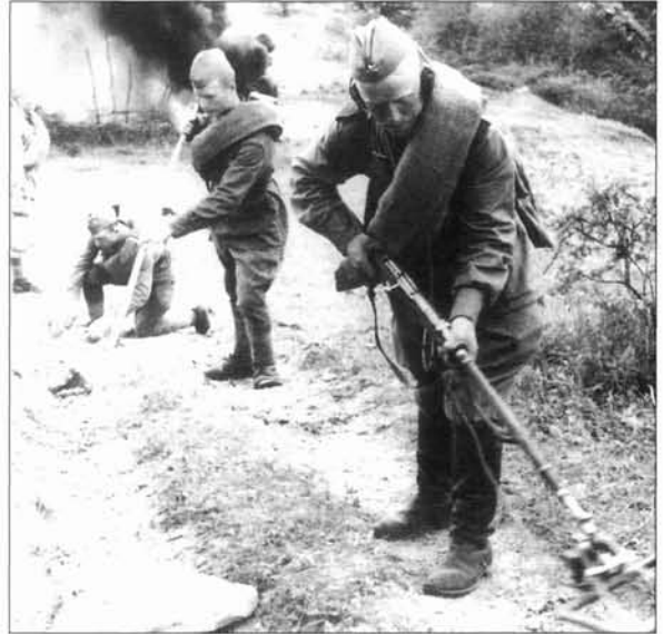
Patrols might be accompanied by specialists to undertake particular missions, such as checking the safety of routes of advance. Here a Red Army engineer searches for mines using a VIM-210 mine detector attached to his 7.62mm Mosin-Nagant M1891/30 rifle; the soldier behind him uses a mine probe – a steel spike fitted to a wooden pole.
