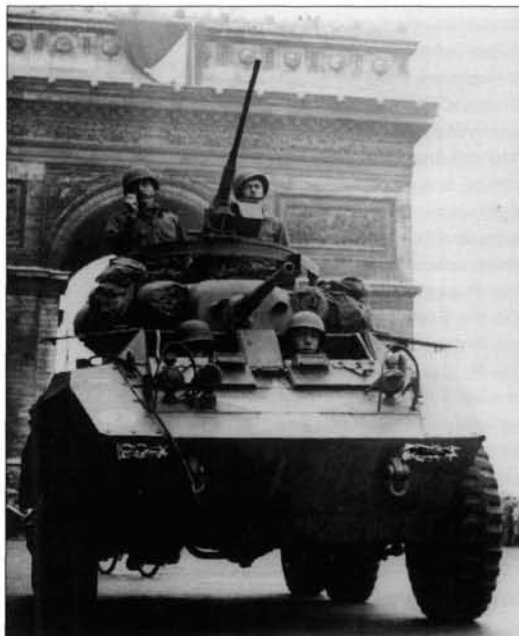
An American M8 Greyhound armoured car in Paris, 1944 – its unit identification bumper numbers have been obscured by the censor. One advantage offered by the armoured cars of divisional reconnaissance units was simply their height (here, 7ft 4in), for better observation and employment of weapons. The M8 was also used by some units of the British Army's Reconnaissance Corps allocated to infantry divisions in Italy.
