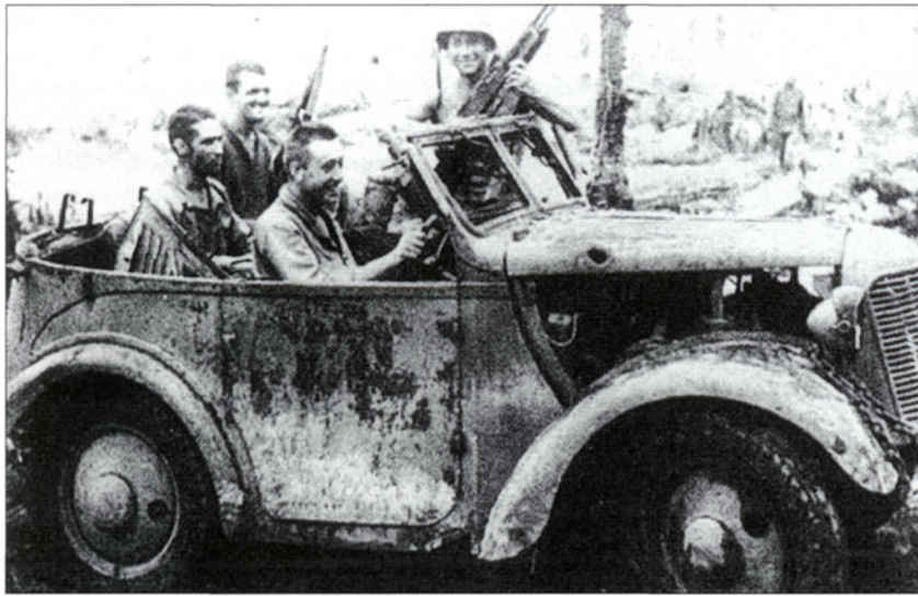
US Marines pose with a captured Nihon Nainenki 4x4 Type 95 (1935) scout car; obviously adapted from a civilian design, this was the Japanese equivalent of the jeep. Like all IJA vehicles, it was in much shorter supply than its equivalents in Allied armies. The Japanese were usually obliged to use foot, bicycle or horsed scouts, and on most Pacific islands they were almost entirely restricted to foot patrolling.
