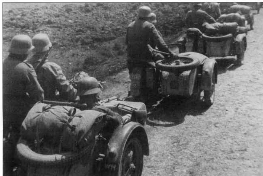
German motorcycle combinations were used to transport machine guns, 5cm mortars, ammunition, and headquarters personnel at platoon and squadron levels. The strapped bundles contain the crew's packs and bedrolls.
