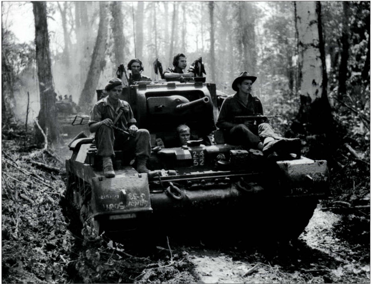
A Matilda tank of 2/4th Armd Regt on the Buin Road, Bougainville, in 1945. Matildas were long obsolete by European standards, and all tanks were restricted by jungle terrain; nevertheless, with their heavy armour and useful 2-pdr gun (or a flame-thrower, in the Mk IV 'Frog' modification), various versions made telling contributions to 'bunker-busting' in Borneo, New Guinea and Bougainville. (Australian War Memorial 092463)
