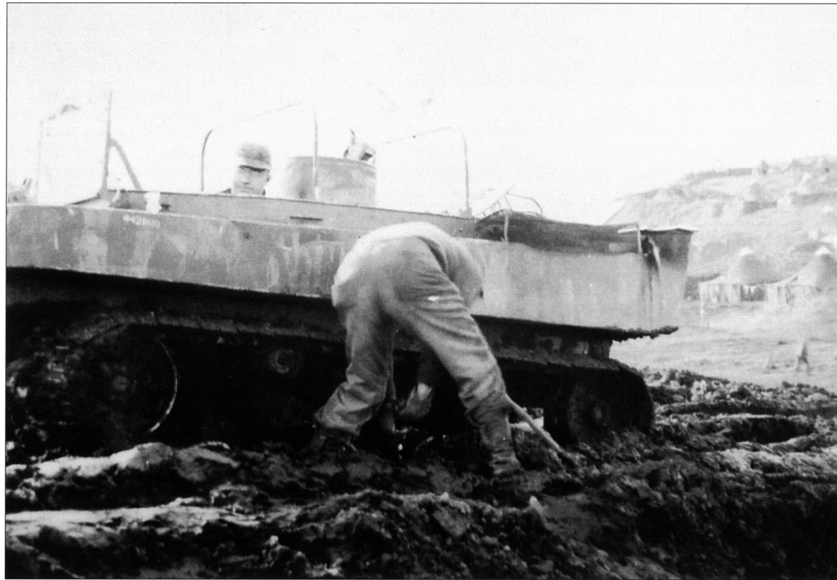
One of the Force's T-15 cargo carriers or Weasels on Kiska. Originally designed for Operation "Plough", the T-15 and later T-24 model went on to serve throughout the US Army after the cancellation of that project. It proved effective in both snow and mud conditions, although its suspension was inadequate to cope with the rocky terrain of the Italian mountains in summertime. (National Archives)
