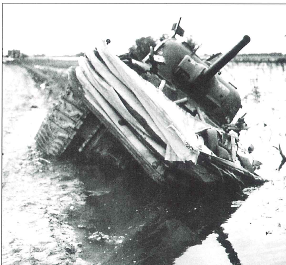
One of the DD Shermans from Co A, 70th Tank Bn was hit by an antitank gun on Exit 2, one of the narrow causeways leading inland through the flooded areas behind Utah Beach. The canvas floatation screen was collapsed around the hull as soon as the DD tanks came ashore; other photos from Normandy show that many crews simply hacked off the skirt at the earliest opportunity. See Plate E.
