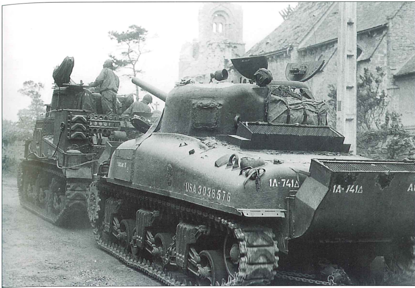
Colleville, Normandy, D+1: an M4A1 still fitted with fording adapters, although the stacks themselves have been jettisoned. This Sherman is A-13, "Adeline II", of Co A, 741st Tank Bn from 1st Armd Div, which supported the infantry of the 16th RCT, 1st InfDiv on Omaha Beach on the morning of June 6. It is seen here being towed by a M31B2 (T2) recovery vehicle after taking a 50mm AT gun hit in the suspension.
