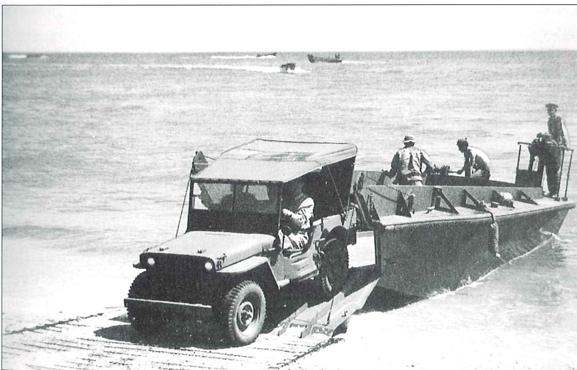
A jeep disembarks from an LCV onto Sommerfield trackway across a beach (see Plate G). The early-war LCV designed by Higgins was the first ramped beaching craft adopted, but it was short-lived. The raised pulpit for the coxswain at the stern meant that such craft could not be stacked or "nested" when stowed aboard transport ships.
