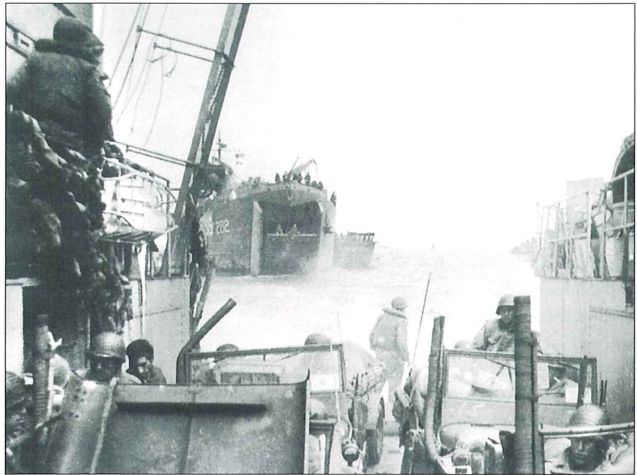
View to stern from an LCT(6) which has just left an LST after embarking a load of jeeps and trailers. The LCT(6) had a removable stern plate; it has been removed from this craft, to allow the vehicles to be driven aboard when the LCT backed up to an LST's bow ramp. The removable plate also allowed LCT(6)s to be lined up bow to stern between an LST and the beach, so vehicles could be driven off over the resultant "causeway" of LCTs.
