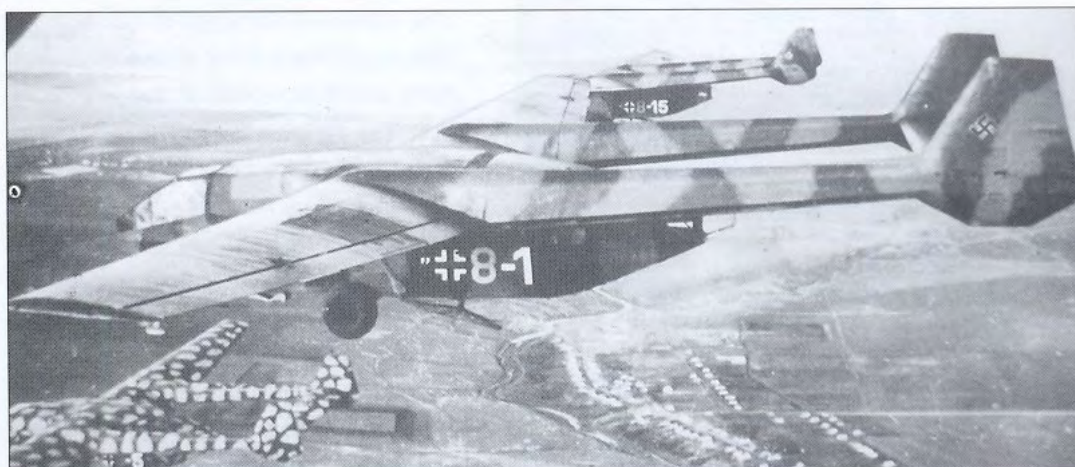
The Gotha Go 242 glider introduced in the mid-war years could carry 21 passengers; but with a tailgate between the twin booms and a payload of almost 5,600lb, it was used almost exclusively for cargo transport. The Germans often used gliders for rear area freight hauling; the Japanese, too, used Kokusai Ku-8 gliders to carry critical equipment and parts from Japan to the Philippines. (Private collection)
