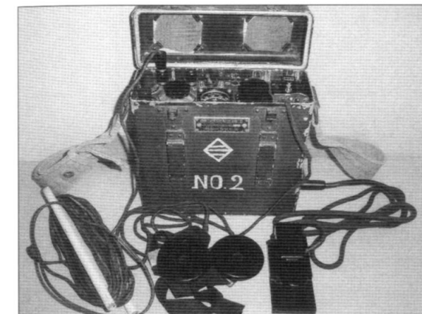
IJN paratroopers required a lightweight radio, but these were not available for the 1942 Dutch East Indies operations. Late that year this experimental set was developed; it did not see use in paratroop operations, but may have been employed by other SNLFs. It measures 8 1/2 x 8 x 2 1/2in, and is painted dark green with white markings. (Yokohama WWII Japanese Military Radio Museum)
