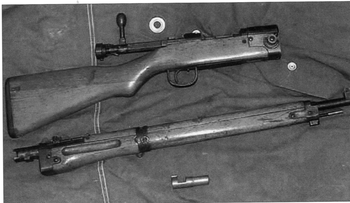
The Arisaka 7.7mm Type 2 (1942) "take-down" rifle, issued from 1943; note the brass muzzle cover. Most Type 2s had a monopod fitted to the forearm, but it has been removed from this example. The unsatisfactory Type 100, which the Type 2 replaced, had lacked the prominent locking pin on the right side of the stock, and the breech portion extending from the barrel was polished. Both rifles were 44in long and weighed just over 8lb 9oz; all Japanese bolt-action rifles had 5-round fixed magazines. (George Kudsus)
