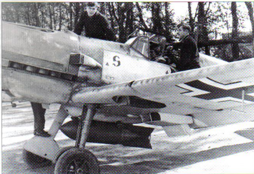
Messerschmitt Bf 109E fighter-bomber of JG 26 carrying a 550-pound bomb under the fuselage. During the final phase of the Battle of Britain, these aircraft made several high-altitude attacks on London. With the small bomb loads and poor bombing accuracy, however, the raids had little effect.
