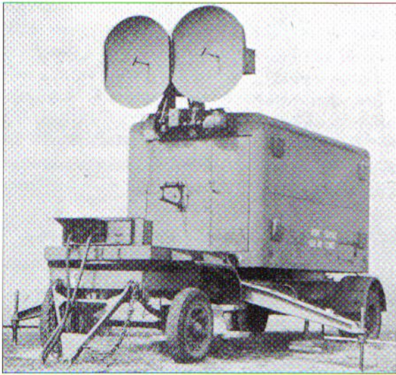
The Gunlaying Mark III radar, designed and built in Canada, brought a major improvement in the accuracy of guns firing at night or through cloud. For the first time, guns could employ continuously pointed fire under these conditions.
