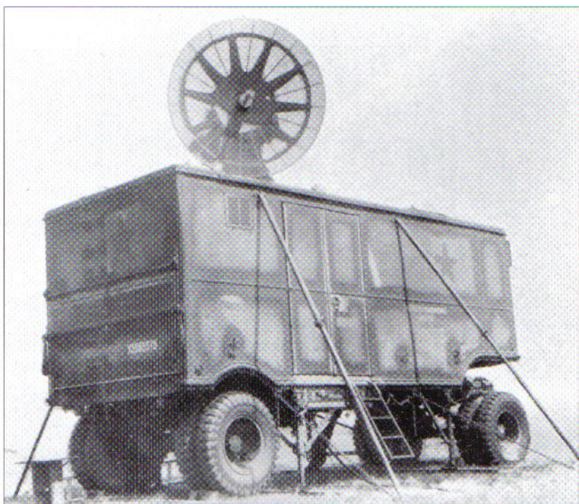
The American manufactured SCR-584 microwave gun-control radar, designated the Radar, AA, No 3 Mark 5 in British Army service. Its use, together with the radar proximity fused AA shell, greatly improved the effectiveness of AA guns against the V.1 missiles.
