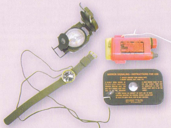
Typical items carried by a LRP, (left to right): Lensatic compass attached to the person by a dummy cord; wrist compass on an olive drab web band carried as a backup; SDU-5E strobe light; Mk 3 signal mirror (backside). (Trey Moore collection)
