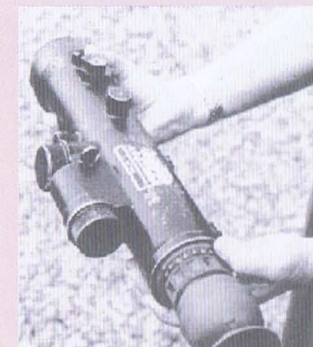
An AN/PVS-1 “starlight scope” that could be mounted on an M14 or M16A1 rifle. These first-generation night vision weapons sights were heavy and of marginal effectiveness. (US Army)
