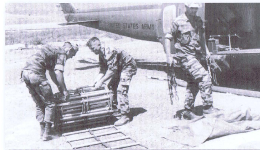
Helicopters were used extensively to insert LRP units into the field. Here troopers prepare an 80ft aluminium rung extraction ladder to rig it into a Huey. The rope woven through the center of the rungs is used to pull the ladder back up. (US Army)
