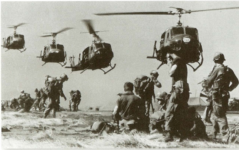
A lift of four Hueys approach a PZ to pick-up their troop loads. The "chalks," the troops assigned to each bird, are formed up to immediately board during a "hot on-load" with engines running.
