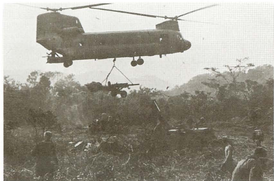
The CH-47A Chinook medium cargo helicopter was the “2½-ton truck” of the helicopter fleet, and was used to carry heavy equipment and supplies as well as troops. Here a “Shithook” delivers a 105mm M102 howitzer to a firebase.
