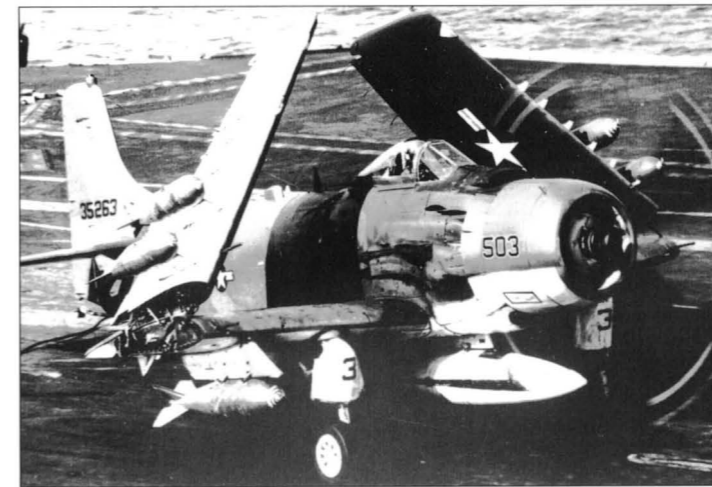
Another of VA-115’s camouflaged A-1Hs taxis toward a catapult on board Kitty Hawk . The black modex ‘503’ is outlined in white for increased visibility. This A-1H (BuNo 135263) is armed with four M117 750-lb low-drag bombs on the outboard wing pylons and 1000-lb low-drag bombs on the two inboard stations (US Navy via Wayne Mutza collection)
