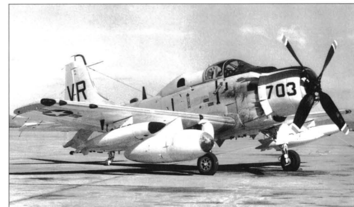
An EA-1F of VAW-13 Det 1 is seen between sorties at NAS Cubi Point on 4 February 1963. The four-seat electronic countermeasures version was known variously as the 'Queer Spad', 'Electric Spad', 'Fat Spad' or 'Left-Handed Spad', the latter because it had only one set of flight controls in the front cockpit. Det 1 supplied the cannon-armed EA-1Fs that flew night intercept patrols in northern South Vietnam during Operation Water Glass in 1962-63 (US Navy via Wayne Mutza collection)
