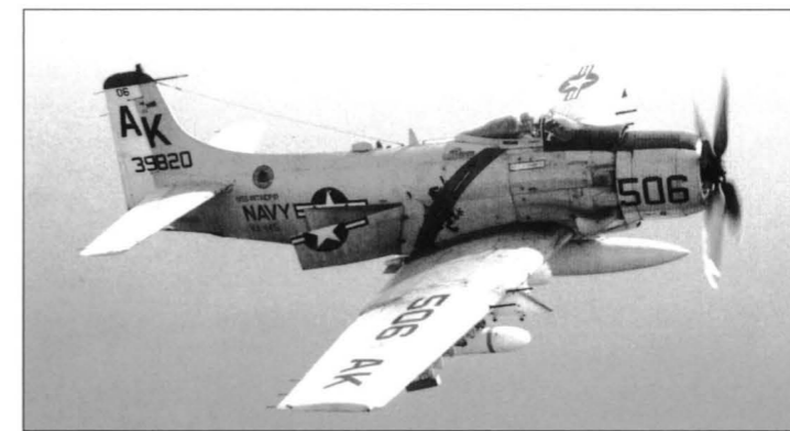
The pilot of VA-145 A-1H BuNo 139820 spreads the aircraft's dive brakes for the benefit of the HU-16 crew it is escorting over the Tonkin Gulf in 1967 during the 'Swordsmen's' last Skyraider deployment to Vietnam. The three hydraulically-powered dive brakes – one on each side of the fuselage and one below – gave the A-1H/J good stability when it came to visually aiming bombs in steep dives (Tom Hansen via Wayne Mutza collection)
