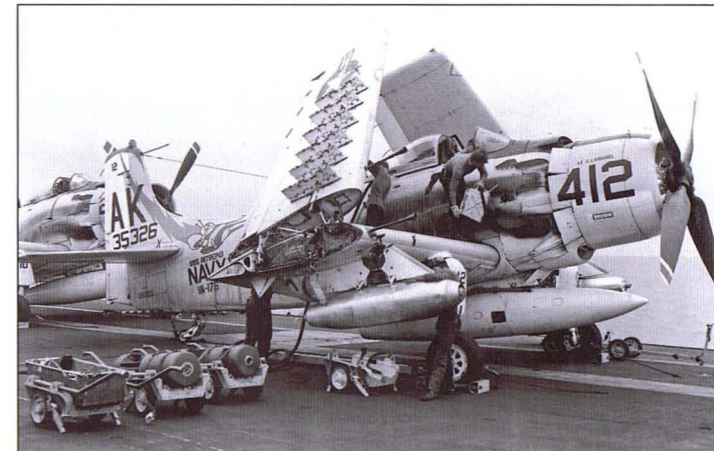
VA-176 A-1H BuNo 135326 is serviced on the deck of CVS-11 in preparation for a mission over Southeast Asia on 20 May 1966. It is armed with Mk 77 mod 1 550-lb napalm fire bombs on the inboard wing pylons. This aircraft was assigned to Lt Charles A Knochel, who was killed in 'Spad' AK 401 BuNo 135239 over North Vietnam on 22 September 1966 - VA-176's only combat loss of the war (US Navy via Robert F Dorr collection)
