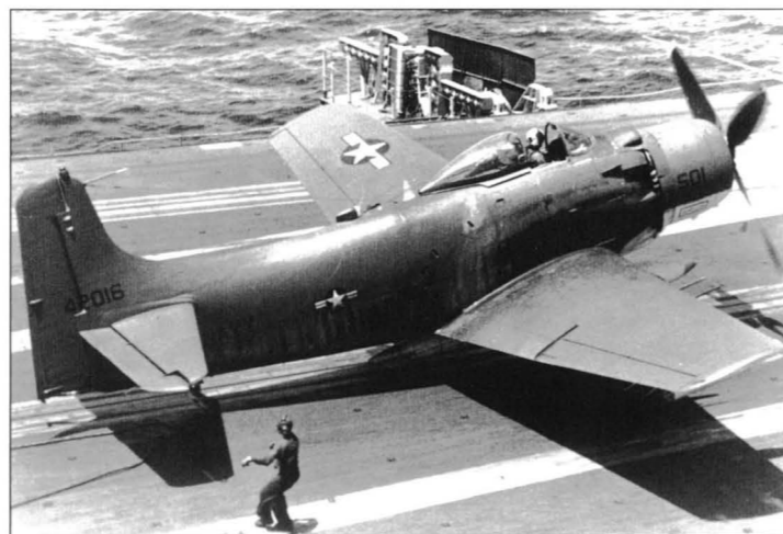
VA-115 A-1J BuNo 142016 taxis forward on the flightdeck of Kitty Hawk on 5 May 1966 as the arresting gear cross-deck pendant retracts. This aircraft was one of several VA-115 Skyraiders that featured experimental water-based paint camouflage applied to its uppersurfaces for the duration of the deployment. The green and olive scheme was abandoned after the cruise. This aircraft was also eventually passed onto the VNAF (US Navy via Robert L Lawson collection)
