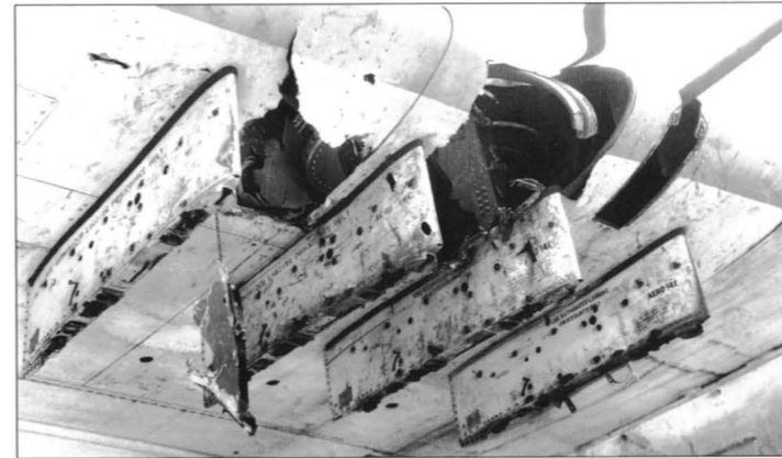
This VA-115 Skyraider recovered at Da Nang AB after receiving damage to its starboard wing during a combat mission over Southeast Asia. The A-1’s rugged construction enabled many shot up aircraft to reach safety. However, a good number of these machines were written off once the damage they had suffered was assessed as being beyond economical repair (USAF via Robert F Dorr collection)
