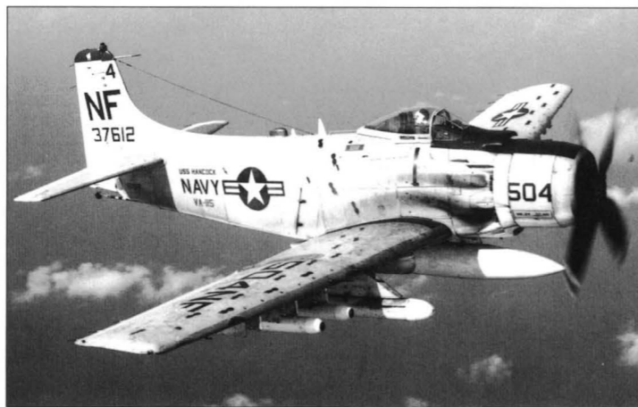
This VA-115 A-1H, seen in the summer of 1967, was assigned to Lt Cdr Jack Jones. It bears one of the more unusual personalised markings seen on a US Navy Skyraider – black-paint footprints of a three-toed person! This aircraft carries seven-shot 2.75-in rockets pods on the outboard wing stations rather than the more common 19-shot pods. Handed over to the USAF following its retirement by VA-115, BuNo 137612 was shot down over South Vietnam on 5 May 1968 and its pilot, Capt Lyn D Oberdier, killed (Tom Hansen via Wayne Mutza collection)
