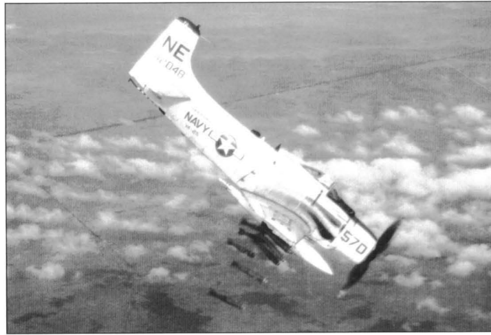
A-1J BuNo 142048 of VA-25 drops a stick of 12 250-lb Mk 81 general-purpose bombs on a Viet Cong target northwest of Saigon in 1965 during the first Vietnam deployment of CVW-5 and CVA-41. Early in the conflict, it was common for carriers arriving in-theatre to conduct combat missions over South Vietnam to season the pilots with light opposition before they were launched over North Vietnam, and its dense air-defence network (US Navy)
