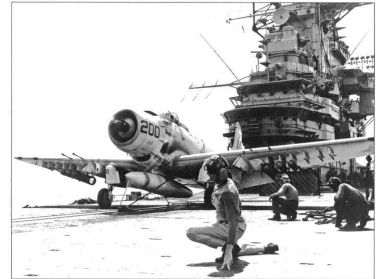
A VA-165 A-1 receives the launch signal from the catapult officer on board CVA-43. As denoted by its modex (NL 200), this aircraft was assigned to the commander of CVW-15. The aircraft is unusual in that it is equipped with a gun camera, located between the starboard landing gear and the starboard inboard wing pylon. Note also the Mk 54 350-lb depth bombs (with ringed tail fins) on these first outboard wing stations. These were frequently used against land targets (US Navy/PH3 Koennenbecker)
