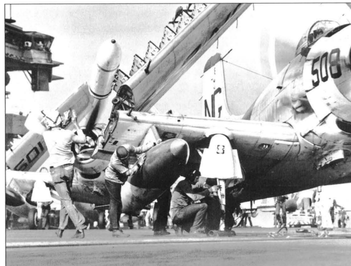
Deckcrewmen perform checks on the landing gear and external fuel tank of a VA-95 A-1 aboard Ranger in the Tonkin Gulf on 24 March 1965 as the 'Spad' is readied for launch. VA-95 participated in the first strikes of the Flaming Dart and Rolling Thunder campaigns against North Vietnam. The 1964-65 cruise aboard CVA-61 was the only Skyraider deployment made by the 'Green Lizards' to Vietnam (US Navy via Robert F Dorr collection)
