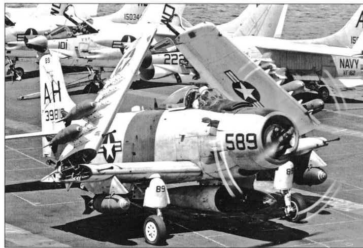
VA-152 A-1H BuNo 139810 taxis toward a catapult past F-8E Crusaders of VF-162 and VMF(AW)-212 on the deck of Oriskany . The 'Spad' is armed with two 1000-lb box-fin bombs and four 500-lb low-drag bombs. The employment of large bombs by A-1 units was common in 1965-66 until the growing SAM threat discouraged the use of Skyraiders on strike missions against targets in North Vietnam (Gary Gottschalk via Wayne Mutza collection)
