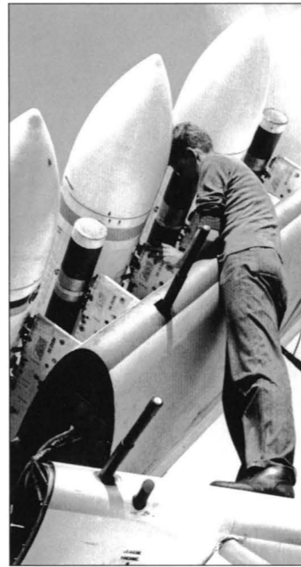
An ordnanceman checks the payload of a VA-95 A-1 on board Ranger on 24 March 1965. This view of the starboard wing shows two M3 20 mm cannon, three Aero 7D 19-shot 2.75-inch rocket launchers and three Mk 24 illumination flares (US Navy/PH1 Moesser)
