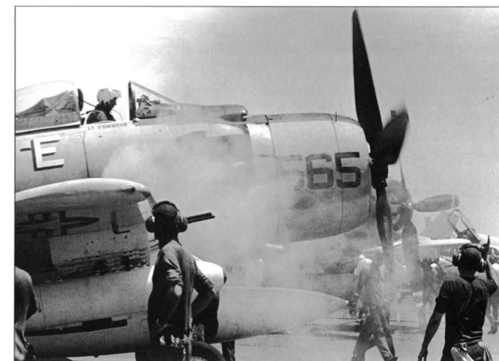
A VA-215 pilot starts the Wright R-3350 radial engine on the deck of Hancock in 1966. The powerful engine enabled the A-1 to carry the ordnance loads for which it is famous. The Battle Efficiency 'E' awarded to the squadron is displayed beneath the cockpit of this aircraft (US Navy)
