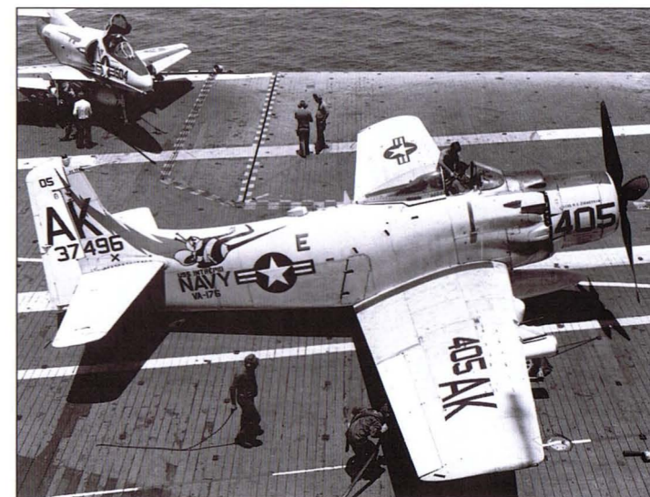
VA-176 A-1H BuNo 137496, assigned to Lt Cdr W C Zimmerman, is refuelled for a launch from CVS-11 in September 1966. The diving bee marking on the empennage became the most famous US Navy Skyraider unit marking of the war (US Navy/AN J A Bahrs via R F Dorr collection)
