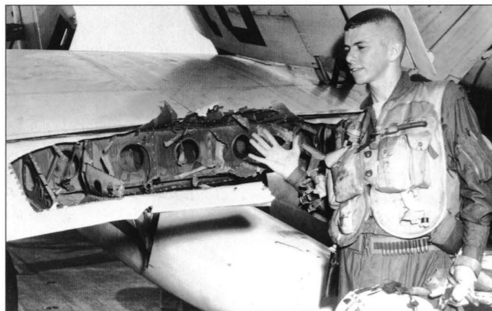
An unnamed VA-165 pilot examines the flak-damaged starboard wing flap of his A-1 on the deck of CVA-43 following a Rolling Thunder strike on 2 April 1965. The pilot is wearing his 'Mae West' life preserver and a pistol belt with a bandolier of bullets (US Navy via Robert F Dorr collection)
