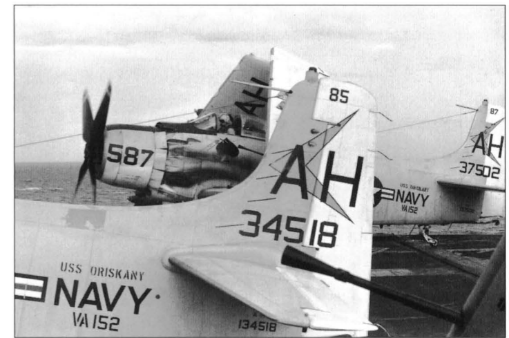
Two A-1Hs from VA-152 prepare for launch from Oriskany in 1965. This photograph clearly shows the typical markings layout for US Navy Skyraiders of the era. The carrier and squadron designation were applied above and below, respectively, the NAVY titling. The last five digits of the six-digit Bureau Number were applied in large numerals on the tail below the carrier air wing tail code (AH for CVW-16). The type designation A-1H and the full bureau number were applied in small letters below the horizontal stabiliser. The last two digits of the nose number, or modex, were applied in small numbers at the tip of the rudder. The rotating beacon at the top of the vertical stabiliser can be used as a date marker for Skyraiders, as they were progressively installed on A-1s in the 1965-early 1966 timeframe. BuNo 137502 was supplied to the VNAF following the completion of its service with the US Navy (Gary Gottschalk via Wayne Mutza collection)
