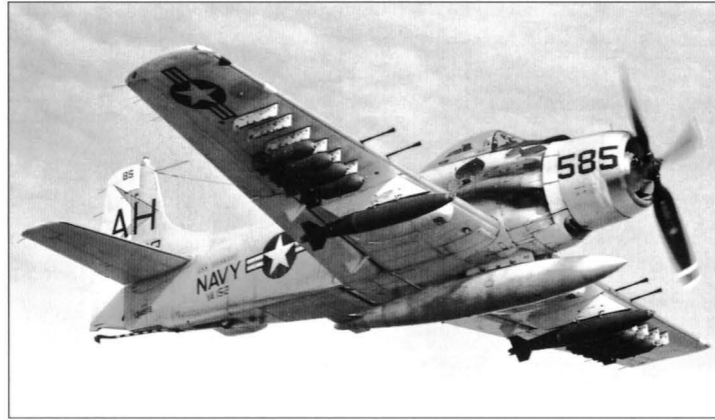
VA-152 A-1H BuNo 134518 presents a warlike pose en route to a target in Southeast Asia in 1965. This 'Wild Ace' 'Spad' is armed with two 1000-lb Mk 83 and four 500-lb bombs. (Gary Gottschalk via Wayne Mutza collection)
