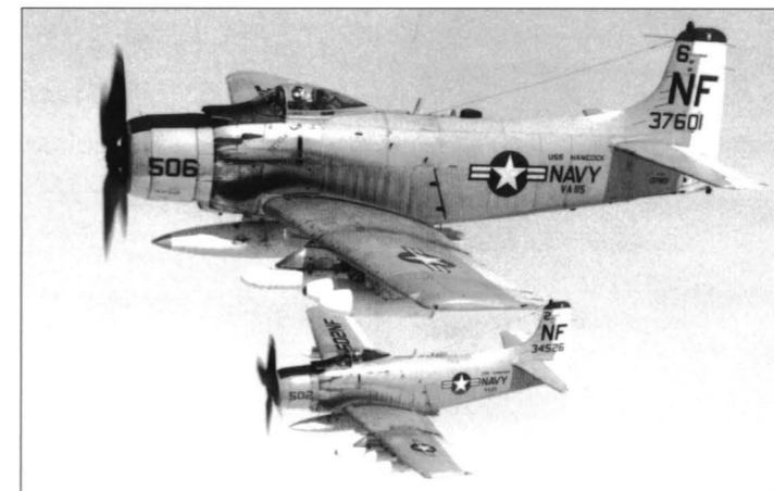
Two VA-115 A-1Hs fly wing on a USAF HU-16B Albatross amphibian, from which this photograph was taken, in 1967 during the ‘Arabs’ second Vietnam deployment, this time with CVW-5 on board Hancock . The aircraft are each armed with two pods of four 5-in Zuni rockets and four 19-shot pods of 2.75-in rockets – a typical load for a RESCAP. The A-1 furthest from the camera (BuNo 134526) was subsequently transferred to the VNAF (Tom Hansen via Wayne Mutza collection)
