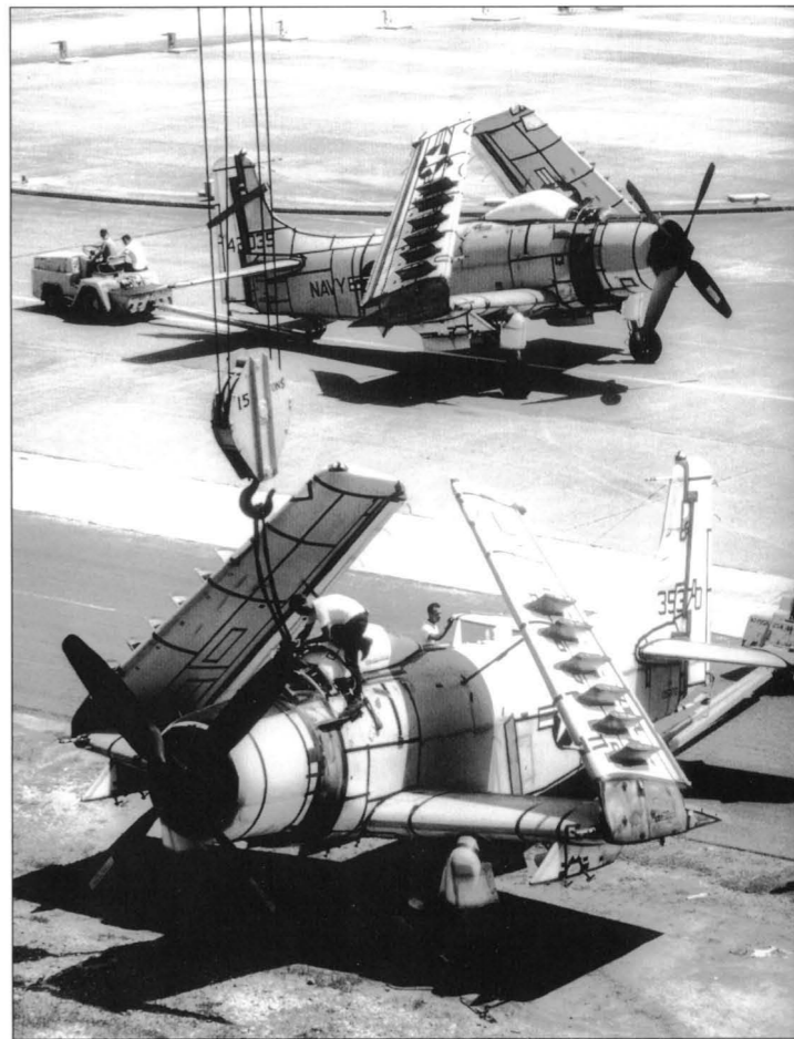
A-1H BuNo 135320 and A-1J BuNo 142039 are offloaded from the aircraft ferry USNS Breton (AKV-42) in March 1966 at NAS Cubi Point, Philippines, where such replacement aircraft were positioned as spares until needed. These Skyriders would eventually replace 'Spads' lost or damaged over Southeast Asia. The aircraft have been sealed with 'Spraylat' to prevent corrosion during storage and transit. Cubi Point, and co-located Naval Station Subic Bay, were the main re-supply and repair bases for carriers and their air wings rotating in and out of the Tonkin Gulf during the Vietnam War. The base complex was a popular rest and recreation respite from the grind of daily air operations over Southeast Asia (US Navy via W M Bowers)
