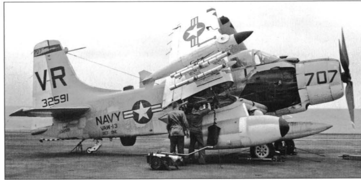
Crewmen service a VAW-13 Det 1 EA-1F on board a carrier in the Tonkin Gulf. An ALT-2/7 jamming pod can be seen beneath the folding section of the starboard wing, outboard of a multiple ejection rack armed with flares. The disc attached to the forward section of the ALT-2/7 pod is unusual, and its purpose is not known. This EA-1F is unusual for a US Navy Skyraider in that a black exhaust mask is painted behind the engine exhaust tubes – a practice common on early A-1Es and A-1Gs in USAF service (US Navy via Robert F Dorr collection)
