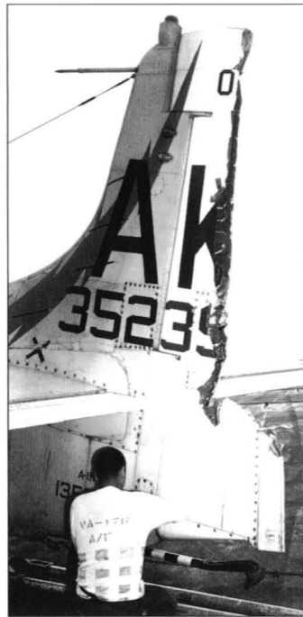
VA-176 A-1H BuNo 135239 had much of its rudder shot away by flak during a mission over North Vietnam. The threat of SA-2 SAMs often drove US aircraft to operate at lower altitudes, where they were vulnerable to radar-guided 37 mm and 57 mm automatic cannons (US Navy/PH3 J A Bahrs via Robert F Dorr collection)
