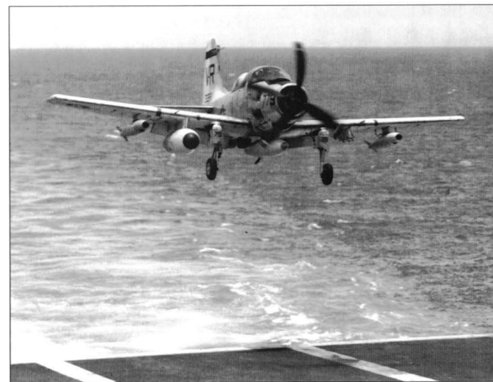
A VAW-13 EA-1F recovers on board CVA-64 on 14 September 1967 after a combat mission in support of strikes over North Vietnam. The fuel dump tube can be seen extending from the underside of the Aero 1C external tank (US Navy/PH2 A P Phillippi)
