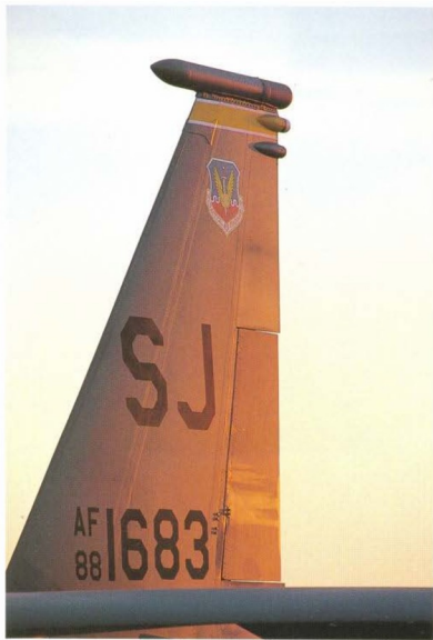
Above left The setting sun picks out all the fine panelling detail on the port fin of a 336th TFS F-15E. The twin rudders on the Strike Eagle are driven by small Ronson rotary hydraulic motors
