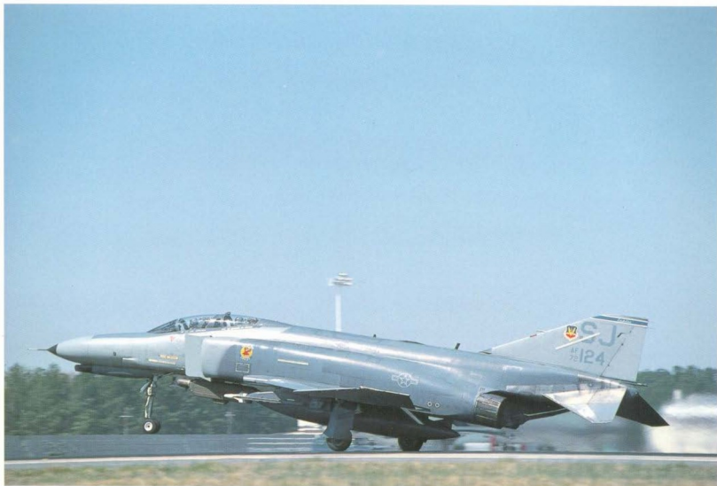
Captured just at the point of rotation, F-4E 72-0124 rockets down the tarmac with its twin J79-GE-17A turbojets on full military power. Besides the mandatory 600 US gal centreline tank and the AN/ALQ-131 ECM pod, this aircraft also carries a single Ford Aerospace AIM-9N Sidewinder round on its port inboard pylon. As with the centre tank, these pylons are always present under the wings of the F-4 and can carry both a TER and a pair of Sidewinders flanking the ordnance
