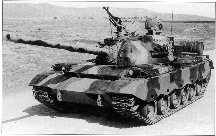
The final evolution of the Chinese Type 59 family was the Type 80. This version used a new suspension based on the American M48 Patton tank and it is armed with a NATO-compatible 105mm gun. (T. Desautels)
