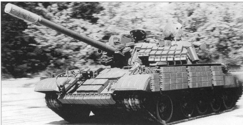
Ukraine was the center for many of the T-55 rebuilding efforts, including the T-55AMV tank with Kontakt reactive armor. This is an example with the full suite of Kontakt reactive armor in place. (Ukrspetseksport)
