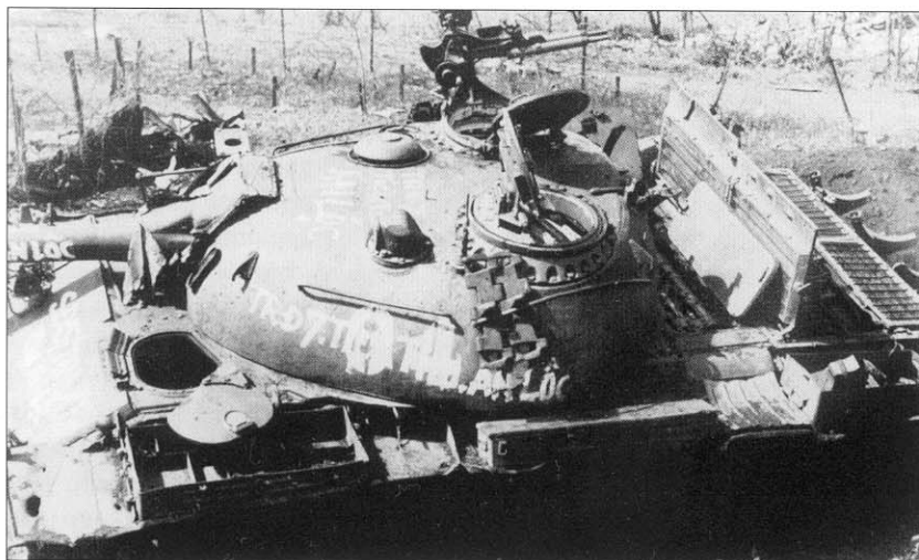
Although most North Vietnamese tank units were equipped with the T-54A or Type 59 tank, a small number of T-54B tanks took part in the 1972 offensive including this tank, probably from the 171st Tank Battalion knocked out at An Loc in April 1972. As can be seen, the tank has the shelf for the Luna searchlight to the right of the main gun, but the searchlight itself has either been knocked off in combat or was left off. (Patton Museum)
