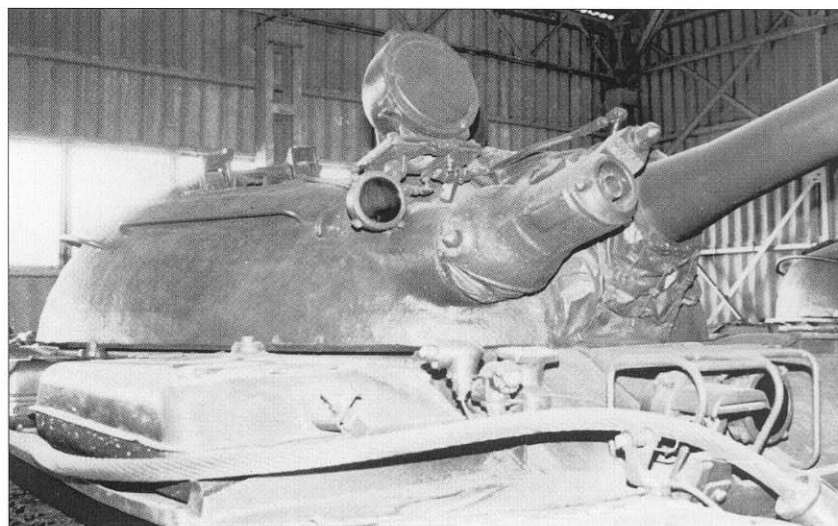
The most widely used of the Soviet flamethrower tanks was the TO-55 ( Obiekt 482 ) based on the T-55. It included an ATO-200 flame-gun mounted alongside the normal 100mm main gun. They were manufactured in 1957-62 on both the T-55 and T-55A, and retired from service in 1993. (S. Zaloga)
