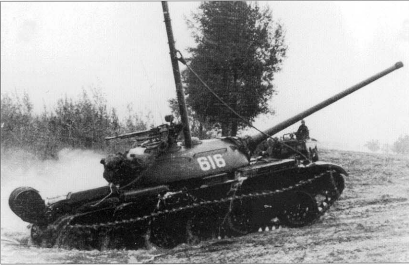
The OPVT snorkel system for deep fording of rivers was added on the T-54A tank. Besides the snorkel itself, the tank had to be extensively waterproofed before the operation.
