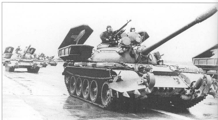
The Polish Army used its own distinctive combat engineer T-55A, fitted at the front with a KMT-4 mine rake, and on the rear with the distinctive bath-tubs containing the PW-LWD rapid explosive breaching system. (Janusz Magnuski)
