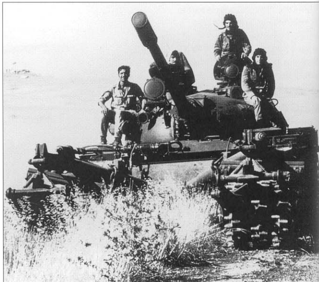
The most common of the T-55 mine trawls was the KMT-5 system. This Syrian T-55 was photographed on the Golan Heights in the wake of the 1973 war after the UN-sponsored ceasefire. (UN)
