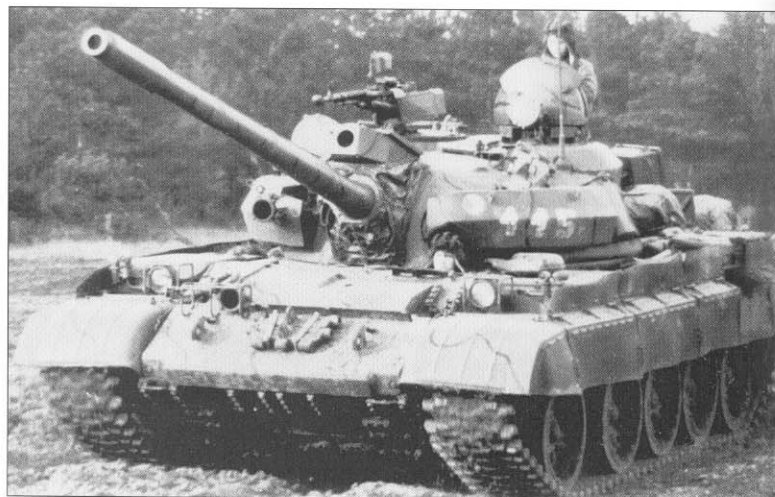
The Czechoslovak T-55AM2 had a number of differences from the Soviet original, most notably the use of the Kladiovo laser rangefinder instead of the Soviet KTD-2, seen here over the main gun. It also used a locally developed wind-sensor on the turret rear, hidden here behind the tank commander. This shows a Czechoslovak T-55AM2 on summer maneuvers in the 1980s in the summer multi-tone camouflage scheme. (US DoD)
