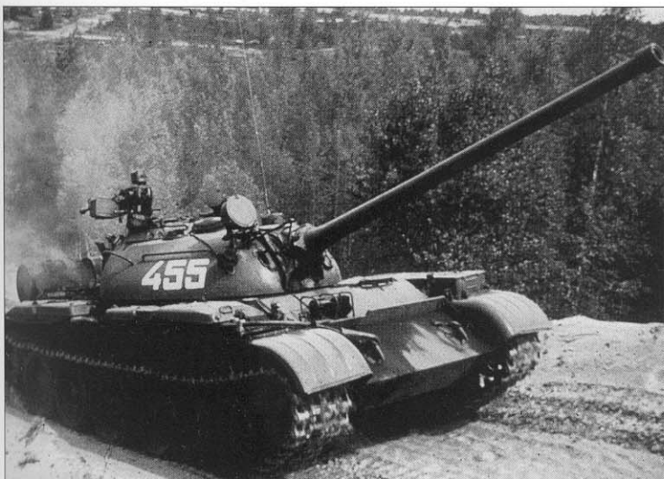
The T-54B introduced the Luna night-fighting system to the T-54 series, most evident by provisions for the L-2 infrared searchlight next to the main gun. In fact, this is a T-54M modernized to T-54B standards, evident from the D-10T gun tube with muzzle counterweight instead of the D-10T2S with bore evacuator that was fitted to the standard production T-54B.
