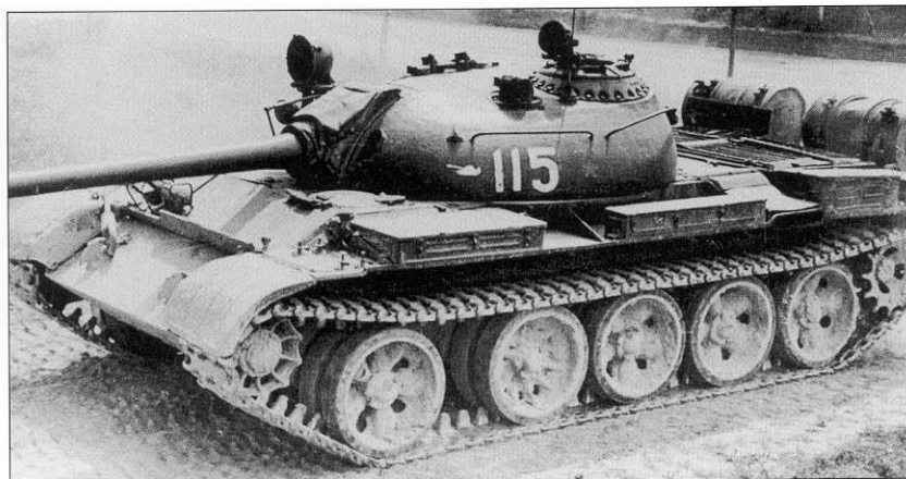
One of the few ways to easily distinguish a T-55 from a T-54B is the absence of the 12.7mm machine gun over the loader and the deletion of the mushroom dome vent on the right roof of the turret. This early production T-55 tank is seen on summer exercise in the early 1960s.
