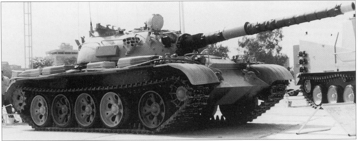
An Egyptian requirement for a large-scale upgrade of its T-55 fleet led to many foreign competitors developing modification kits. This example by Britain's Royal Ordnance substituted the NATO-standard 105mm gun and included many fire control improvements. (C. Foss)
