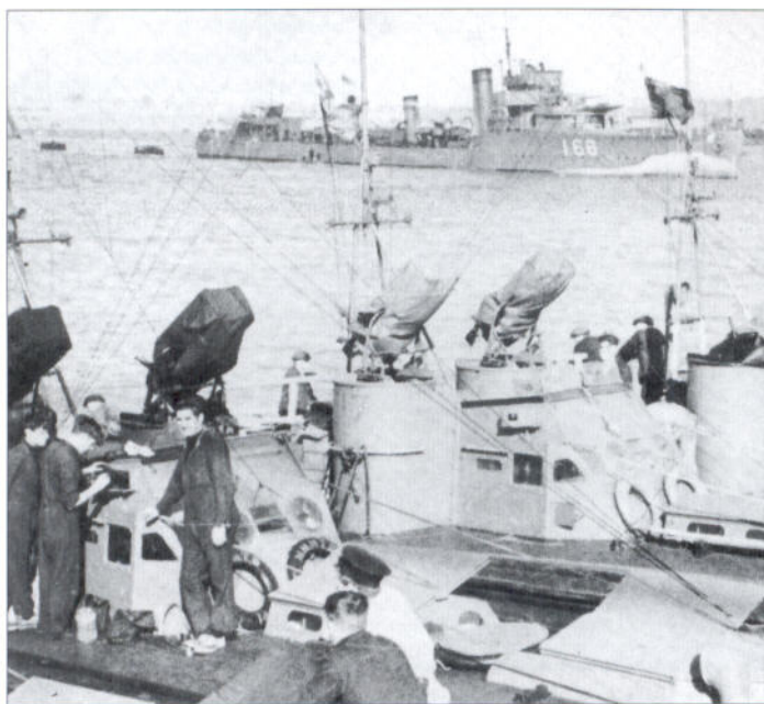
60-foot British Power Boat MTBs at Harwich, 1940, with the escort destroyer HMS Wyvern in the background. Lewis guns were mounted fore and aft, but later, the armament was reconfigured, and the guns were mounted in twin bins on either side of the bridge. (Imperial War Museum)
