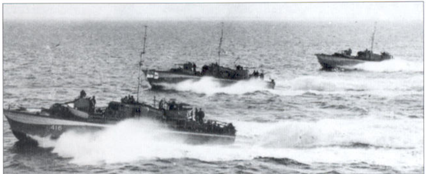
A trio of British Power Boat vessels (MTB 416, 413 and 412, all 71-foot 9-inch Mark V boats) photographed in the English Channel in June 1944. With a powerful armament and a top speed of 39 knots, these were amongst the best-designed MTBs of the war. (Imperial War Museum)
