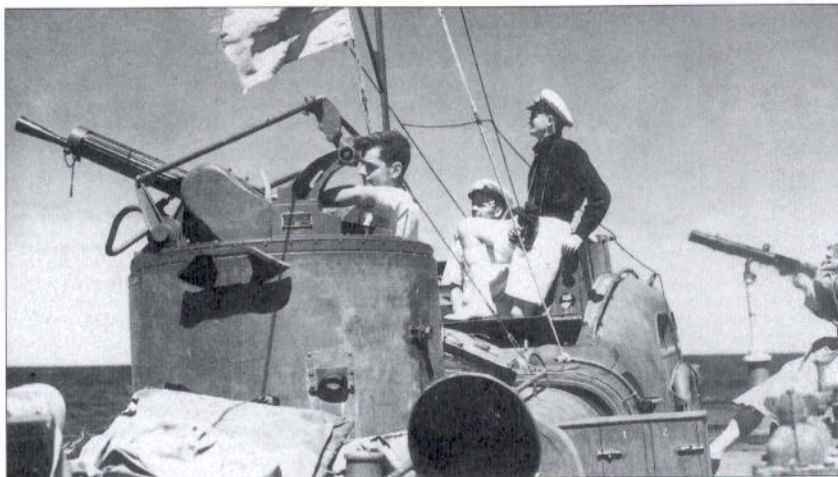
The power-driven mount of a twin .5-inch Vickers machine gun mounted amidships on a 70-foot Elco boat in the Mediterranean. The bin itself remained stationary, and the gun and mounting ring rotated inside the turret. (Imperial War Museum)
