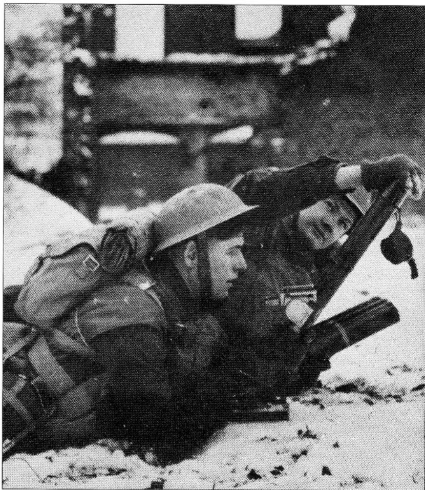
Two British soldiers operating a 2-inch mortar. The firer holds the mortar steady while the other soldier loads a bomb into the muzzle end. Once the bomb has slid down to the breech end of the barrel the firer operates the lever mechanism by means of a short lanyard to 'trip' the firing pin. (MFP)
