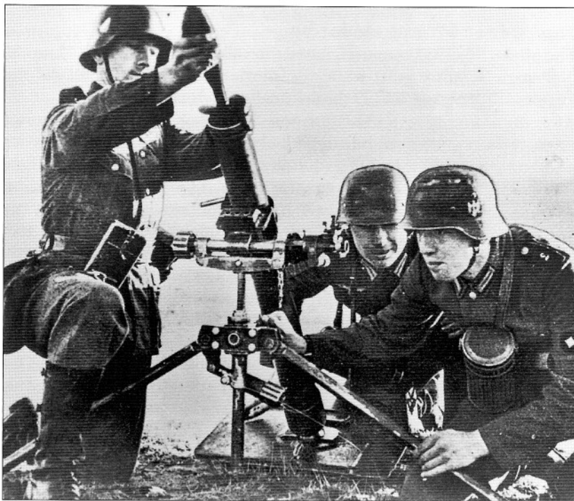
German Army 8cm Granatwerfer 34 mortar in action. The three-man crew are seen variously loading the mortar, checking the sight and steadying the tripod mount. As a support weapon the Granatwerfer 34 was invaluable in providing fire support during assaults and defensive actions. (IWM, STT 3211)
