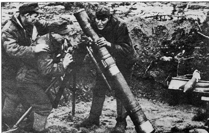
The German Army's version of the captured Soviet 120mm mortar. Known as the Granatwerfer 42 this was virtually a direct copy of the Soviet Army's weapon and intended to capitalise on the huge stocks of ammunition which had been captured along with the original version of the weapon. (IVH).
