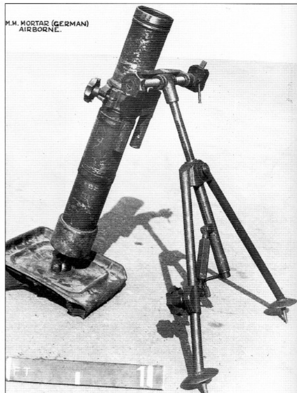
The shortened version of the standard German Granatwerfer 34 as in use with parachute and some specialist infantry units. Despite its reduced range following the change in barrel length, this weapon was well liked by the parachute units who valued it for its firepower and versatility. (IWM, HU22571)
