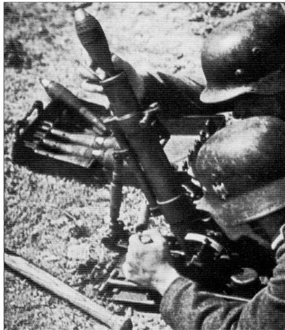
The German 5cm Granatwerfer 36 in action. It is being loaded by the man on the right with the firer making adjustments to range and angle of barrel before actual firing. Note the ammunition container to the middle rear of picture. (MFP)
