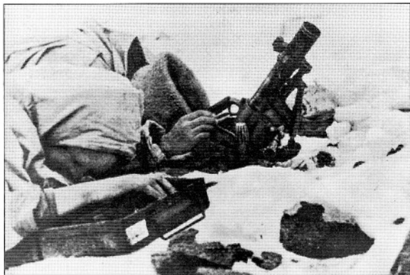
The German Army 5cm Granatwerfer 36 in action. The crew appear to be huddled against enemy fire, an action which emphasises the compact design of the weapon, which had a barrel only 19.3 inches in length. (IWM, STT 5536)
