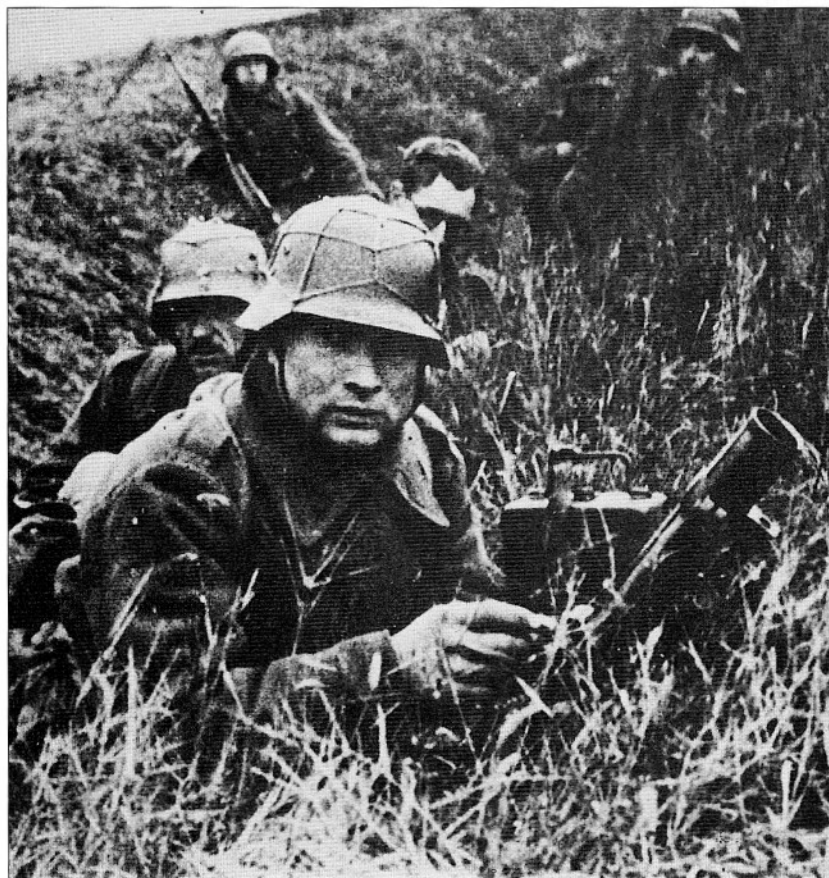
German 5cm Granatwerfer 36 in service with a rifle platoon who are seen just prior to moving forward to make contact with the enemy. With a maximum range of 550 yards this weapon could provide good close-quarter fire support in either the attack or defence. (MFP)
