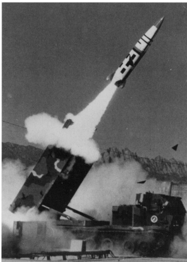
Besides the normal rockets, the MLRS can also carry and fire two of the larger MGM-140 ATACMS missiles, used for deep attack of key enemy positions. The current versions of the missile drop a payload of submunition grenades on the target, but future versions will use the BAT guided submunition. (US Army)
