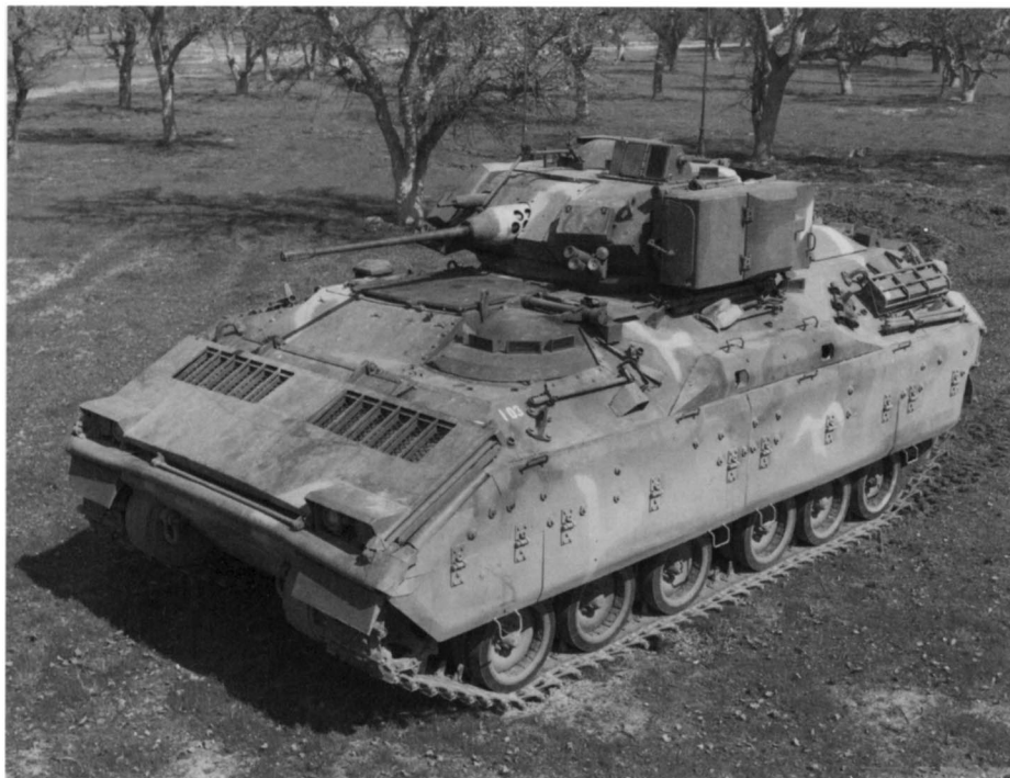
This is one of the pre-series XM2 Infantry Fighting Vehicles showing the new two-man turret with TOW missile launcher. The early test vehicles can be distinguished by the fairing over the side firing ports, a detail that was simplified on the production vehicles. (United Defense LP)
