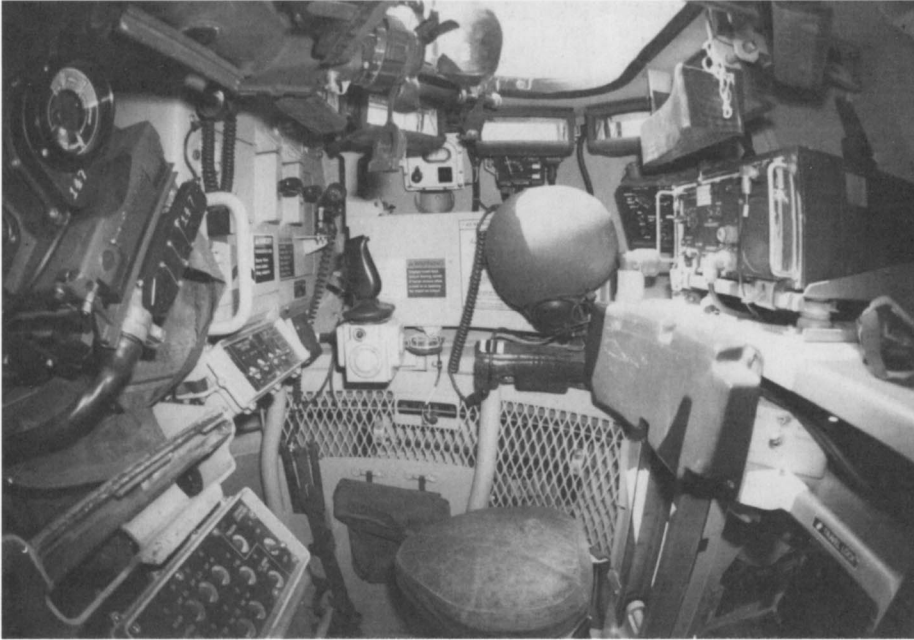
This is a view of the turret from the gunner's side of the turret, looking over to the commander's station on the right hand side. The rear bustle of the turret contains the vehicle radios. While riding inside the Bradley, the commander wears a normal CVC helmet which is attached to the vehicle's communication system. (Author)
