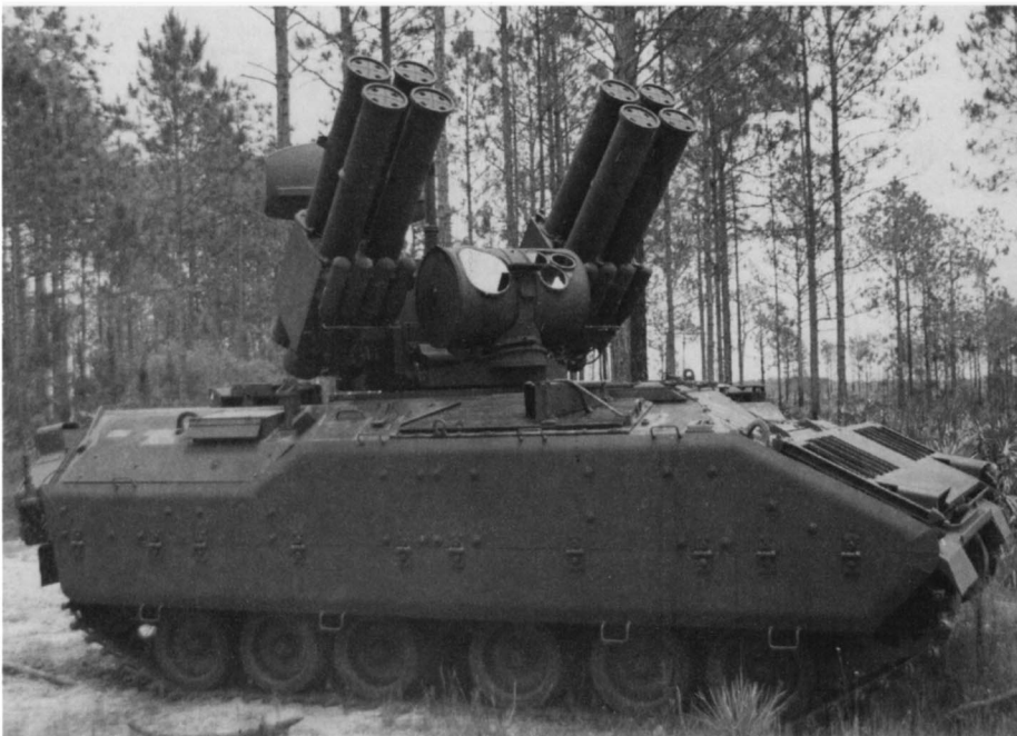
The Bradley was selected as the chassis for the ill-fated MIM-146 ADATS air defense missile system, which was eventually cancelled due to the low priority afforded tactical air defense within the US Army. The system was first deployed in the Canadian Army, but uses a M113 chassis. (Martin Marietta)
