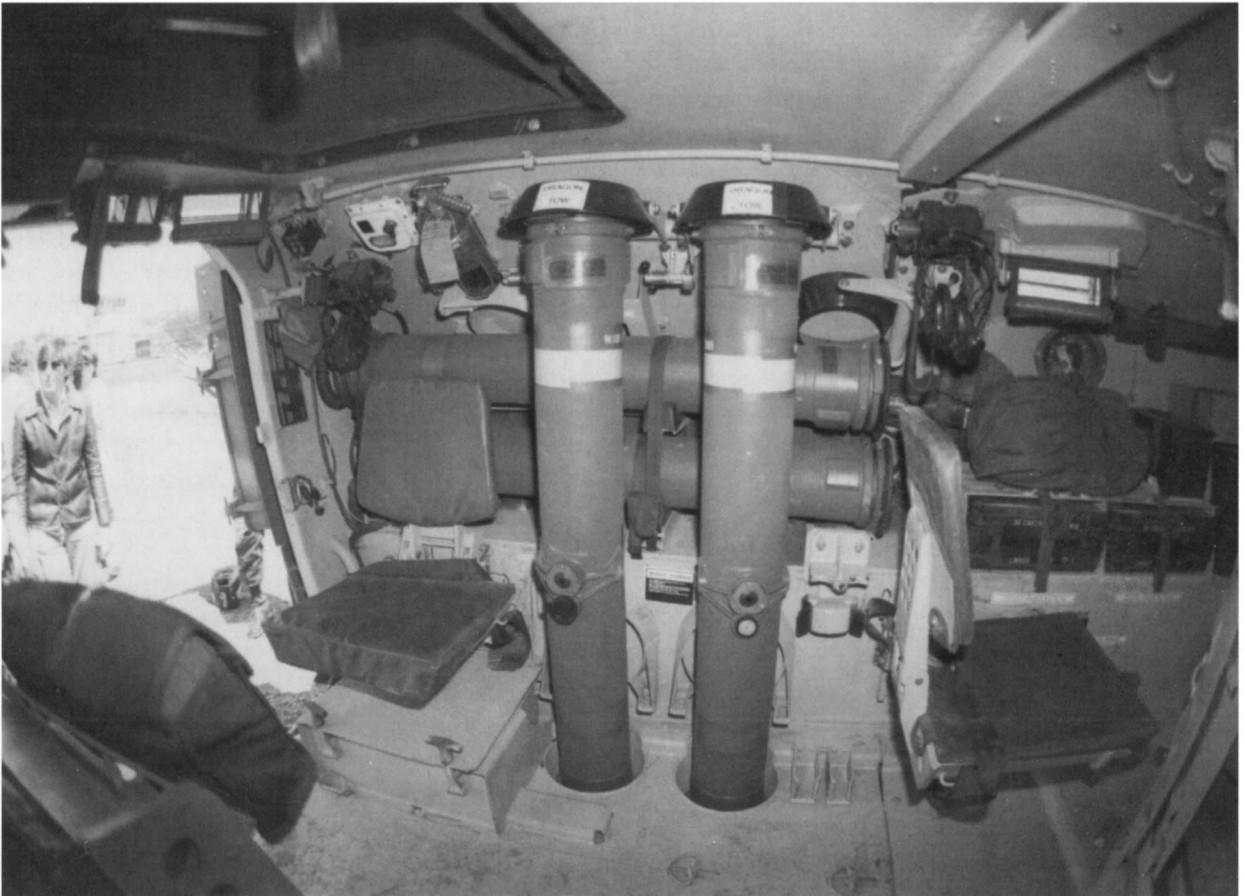
The left hand interior of the M2 Bradley IFV has storage for four TOW or Dragon anti-tank missiles. This places them within easy reach of the crewman in the left rear of the troop compartment for reloading the TOW launcher. (Author)
