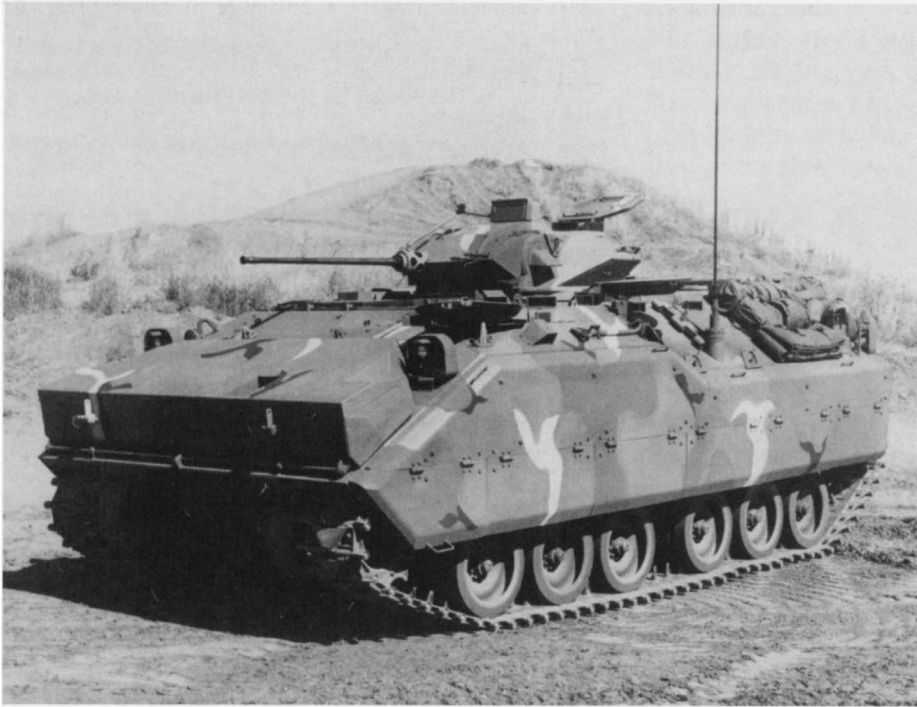
The FMC Corp design, the XM723 MICV, was the forerunner of the current Bradley Fighting Vehicle. The hull configuration is very similar to the eventual Bradley design, but the one-man turret without an anti-tank missile launcher became the centre of dispute between the infantry and cavalry branches. (United Defense LP)
