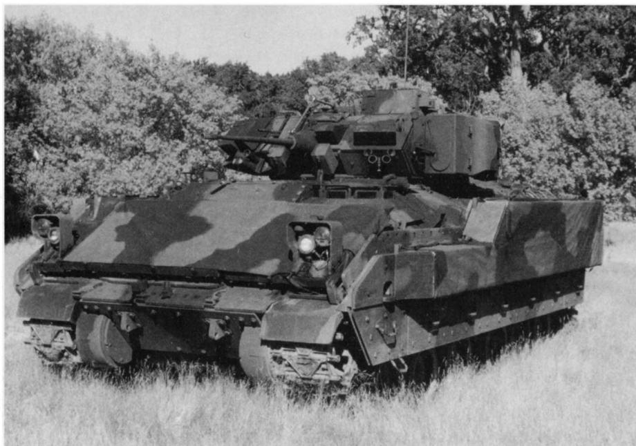
From the outset, the Bradley A2 was designed to accept reactive armour tiles for additional protection against shaped charge warheads such as those found on anti-tank rockets and missiles. Two competitive designs were developed, and in 1993, the Martin Marietta/Rafael design was selected. In the field configuration, the tiles are contained in steel boxes, which are covered with a camouflaged fabric cover. (United Defense LP)
