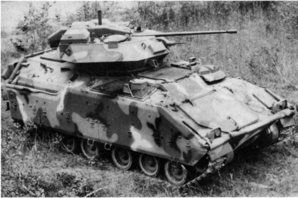
The CVAST was one of the early attempts to up-arm the Bradley to respond to future Soviet infantry vehicle developments. In the event, the new BMP-3 is not well armoured, and the end of the Cold War has pushed the follow-on COMVAT programme into a low-priority slot. (United Defense LP)
