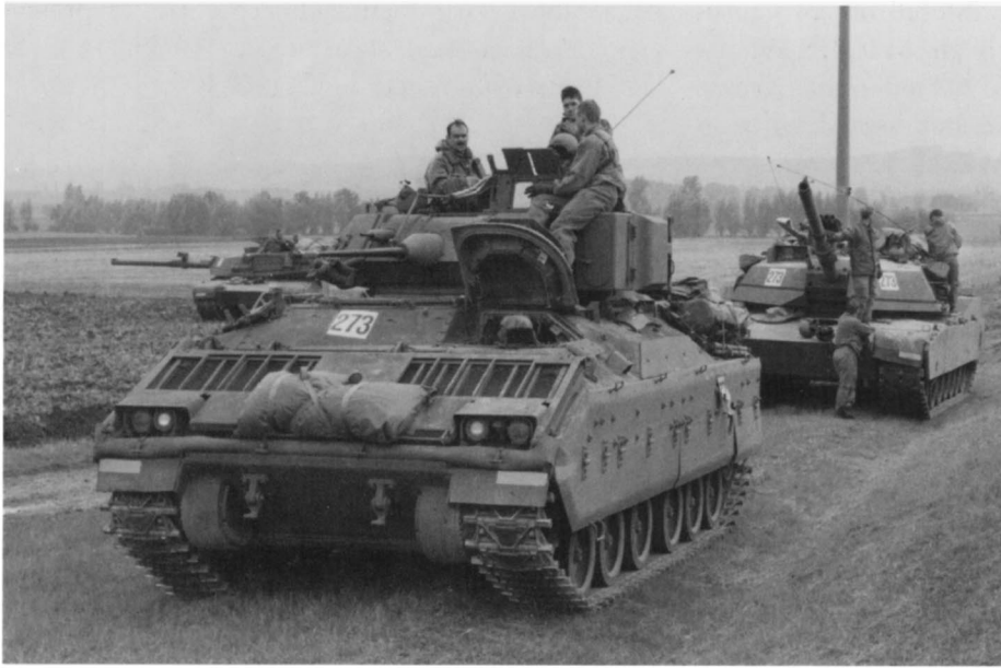
A M3A1 CFV leads a column of M1 Abrams tanks during a field exercise in Germany in 1989. A careful inspection of the side plate below the TOW launcher will reveal the absence of firing ports on this vehicle, a sure sign that it is a Cavalry Fighting Vehicle. (Pierre Touzin)
