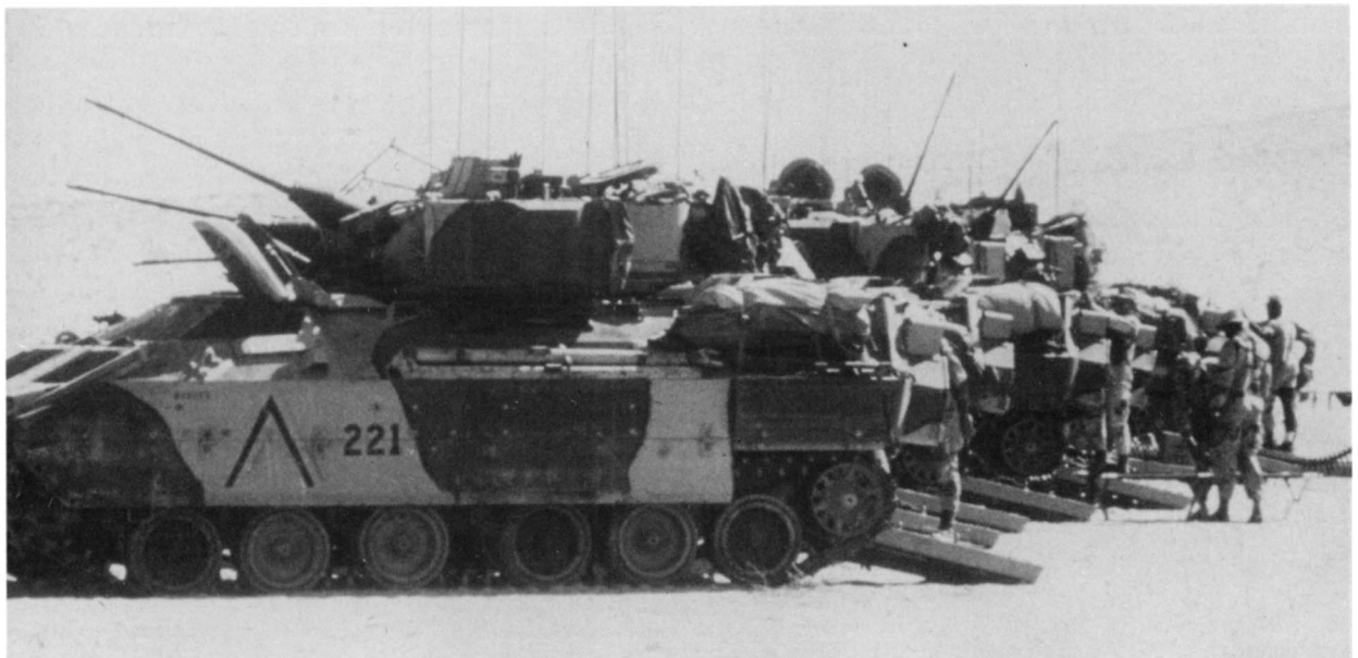
M3A1 CFVs of the 1-4th Cav., 24th Inf. Div. (Mech) in Saudi Arabia before the outbreak of the ground campaign against Iraq, the vertical rear storage bins are a characteristic feature of this version; the first 284 Bradley A1s still had the angled rear turret bins. This unit was one of a few US Army units to pattern paint camouflage during 'Desert Storm' - the other battalions of the division all used the normal overall CARC tan scheme. (Frank DeSisto-Intrepid Museum)
