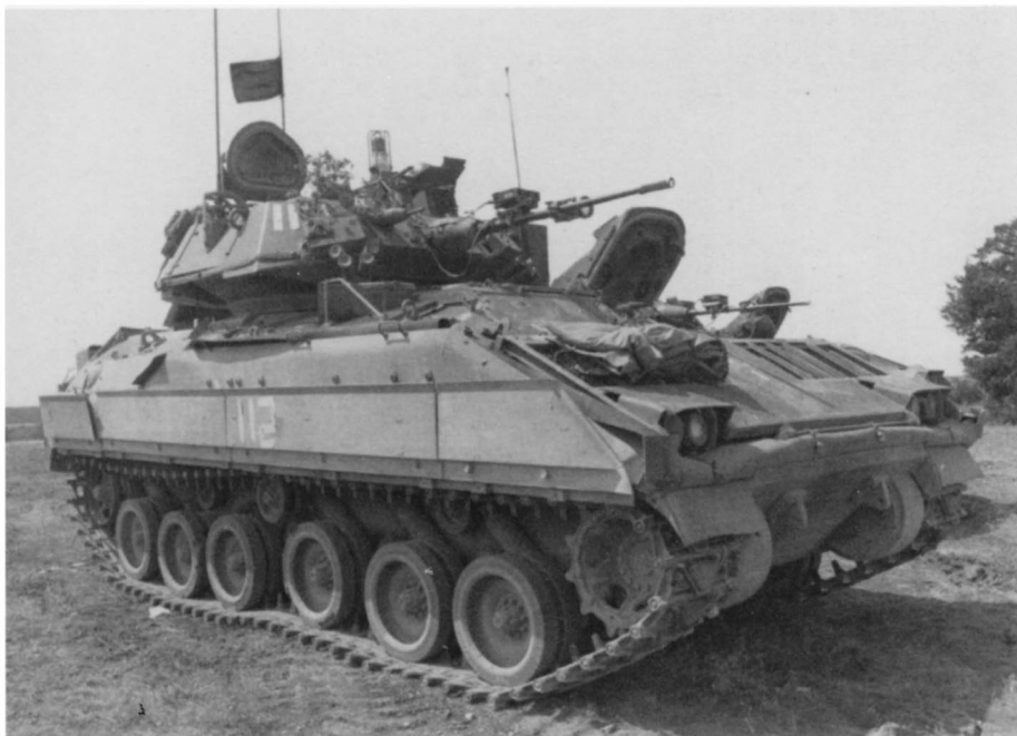
An M3 CFV of the 1st Cavalry Division during exercises at Ft. Hood Texas in 1987. During the production of the Bradley, a continual series of small improvements were added to the vehicle, such as the guard placed at the base of the turret radio antenna to prevent it from being broken by crewmen climbing into the turret. The crews at some posts operate the Bradley with the lower track raised since it eases track maintenance. In the case of this Bradley, the vehicle tactical number, 112, has been added on the inside of the skirt in reflective tape. (Author)
