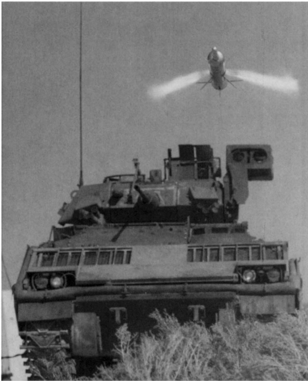
The merger of the infantry and cavalry requirements led to the addition of a TOW anti-tank missile on the vehicle. This dramatic view shows a BGM-71C Improved TOW shortly after launch with its two lateral rocket motor exhausts in full thrust. The TOW has undergone continuous evolution to keep up with advances in tank armour, and the Bradley A1 series was developed to take advantage of the BGM-71D TOW-2 missile. (Hughes Missile)
