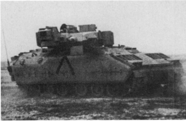
This rare shot shows one of a handful of Bradleys fitted with the VLQ-7 Stingray electro-optical jammer deployed to Saudi Arabia for 'Desert Storm'. This medium energy laser device was designed to blind electro-optical sensors such as tank sights, and was fielded as a possible response to Iraqi use of lasers to blind troops.
