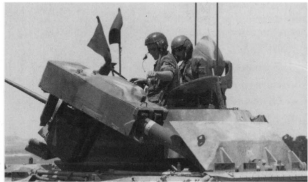
The large hatch on the rear deck of the Bradley is used when reloading the TOW launcher. The hatch is designed to partially open, minimising the exposure of the crewman to hostile fire while reloading. (Author)
