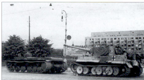
A turretless KV-1 being used as a recovery vehicle tows a captured Tiger 1 heavy tank across Revolution Square in the Petrogradskiy section of Leningrad in 1944.
