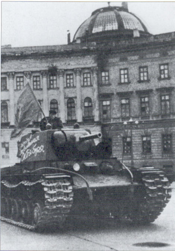
The April 1941 'gun scare' led to the development of an up-armoured turret for the KV-1, which began to be manufactured in the summer of 1941. This is a tank straight from the Kirovskiy Plant in Leningrad, being sent to the nearby front to defend the city in the autumn of 1941 shortly before the plant was evacuated. The political slogan on the turret side reads 'We defend the Conquests of October', referring to the 1917 Bolshevik revolution in the city.
