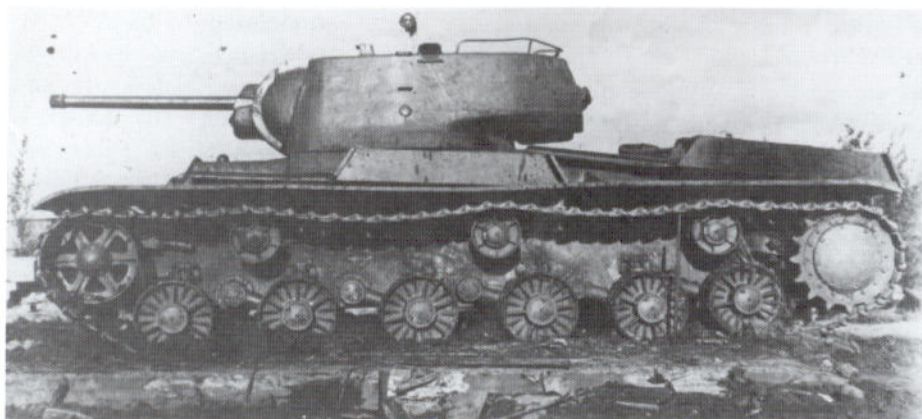
In 1942 there were some experiments to mount artillery rockets on tanks such as this KV-1K. Two armoured boxes were fitted on the fenders, each containing two rail launchers for RS-82 Katyusha rockets. Ultimately, this idea was dropped, probably due to the inaccuracy of the rockets. (R. Ismailov)
