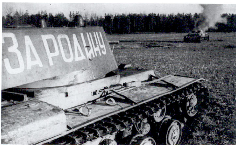
A colourfully marked KV-1 Model 1941 moves forward past a smouldering German PzKpfw IV on the Southwestern Front in 1942. This is one of the original KV-1 Model 1941 configurations with the early pattern welded turret, early style resilient roadwheels, and the initial pattern turret ring appliqué. The slogan on the turret is Za Rodinu – 'For the Homeland'.
