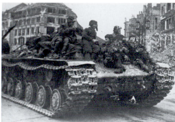
Some old KV hulls continued in service right through the to end of the war. With its turret removed, this KV-1 Model 1940 is being used as an armoured recovery vehicle to tow a disabled T-34-85 in the wreckage of Berlin in
