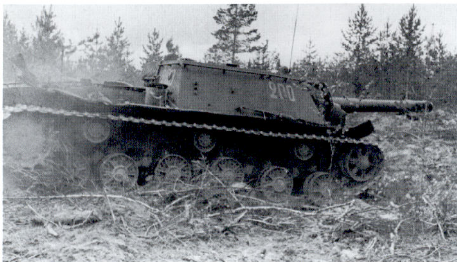
The SU-152 proved very successful; in 1943 it was one of the few armoured vehicles in the Red Army that could stop a Tiger or Panther, earning it the nickname Zvierboi ('Animal Hunter'). This is another view of the SU-152 of Lt. Berezin on the 2nd Baltic Front in 1944. By this time the improved ISU-152, on the new IS-2 Stalin chassis, was entering service. (Soloviev)
