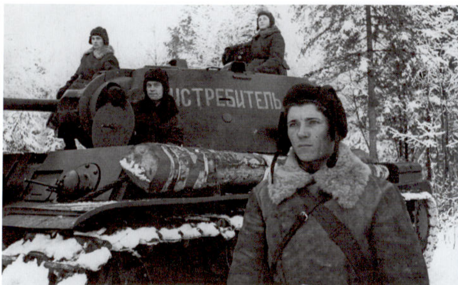
The crew of a KV-1 Model 1941 (cast turret) tank named Istrebitel ('Fighter') on the Kalinin Front in northern Russia in the winter of 1942. The tank commander, Jr. Lt. I.M. Tovstikh, is in the foreground. The tank is carrying a large piece of timber, which was used as an unditching beam to extract the tank from soft ground. (P.I. Maksimov)
