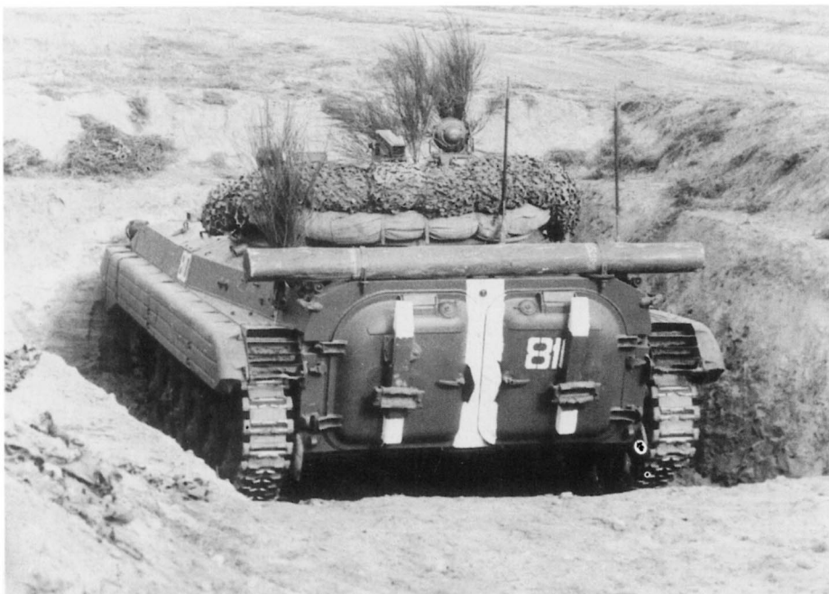
The BMP-2K is a company command version of the BMP-2. It is similar in appearance to the basic version, but has an additional radio mast at the rear as seen here, and lacks the full set of firing ports on the hull side. The white band insignia indicates a vehicle participating in autumn wargames with the aggressor forces. (US DIA)
