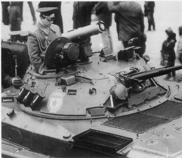
The BMP-2 was subjected to a number of improvements during its manufacture. By the early 1980s, a layer of lead-impregnated armour was added to the turret sides to provide additional anti-radiation
