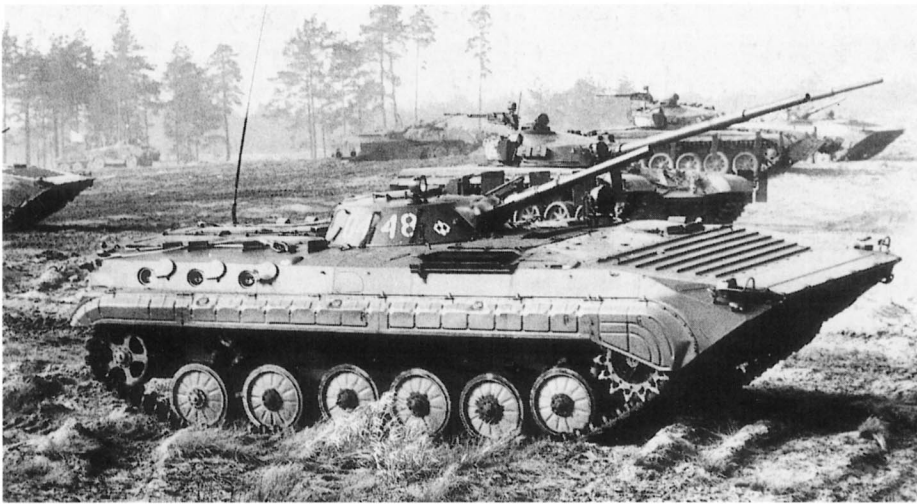
The BMP-1 was widely exported to the other Warsaw Pact countries, and Czechoslovakia eventually undertook local manufacture. Here, a Polish BMP-1, locally known as the BWP-1, takes part in exercises with the T-72 tanks of a Polish armoured division in western Poland. Note that the side firing ports are open, although the AKM assault rifles do not appear to be fitted.
