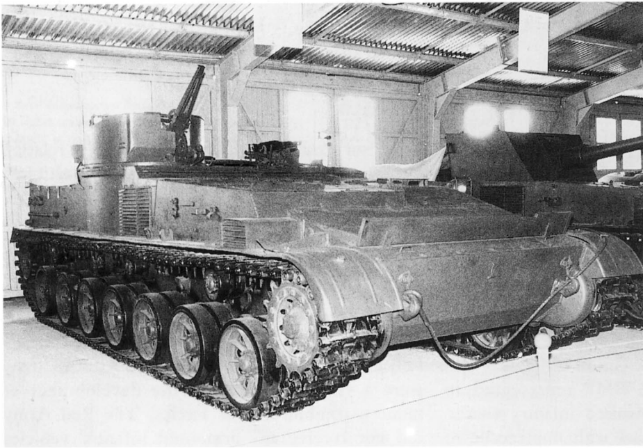
The first serious attempt at developing a tracked infantry vehicle in the USSR was Gorlitskiy's Obiekt 112. This was designed to carry 25 infantrymen and was armed with a heavy machine-gun in the pulpit on the right. It proved too expensive and complicated for the Red Army in 1949, but served as the basis for the 2S3 Akatsiya, 2S4 Tyulpan and 2S5 Giatsint SP artillery vehicles.
