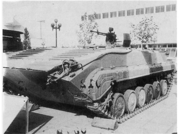
The Chinese WZ503 series is based on the BMP-1 hull, but has had the side panels heightened to provide more
