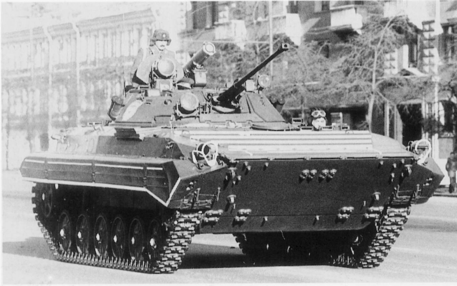
The design finally selected for the BMP-1 replacement was the Obiekt 675, which mounted the new Shipunov 2A42 30mm autocannon in a new full-profile, two-man turret on a standard length BMP hull. This vehicle was designated BMP-2 on entry into service in 1977. The fenders were widened to accommodate floatation cells since the new turret's additional weight affected the bouyancy of the vehicle when swimming. (US DIA)
