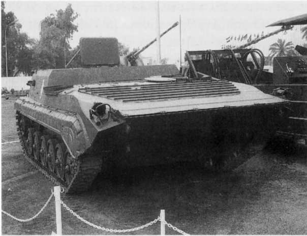
The Iraqis converted a number of BMP-1s to armoured ambulances by the addition of a fixed superstructure to the hull rear. A small number of
