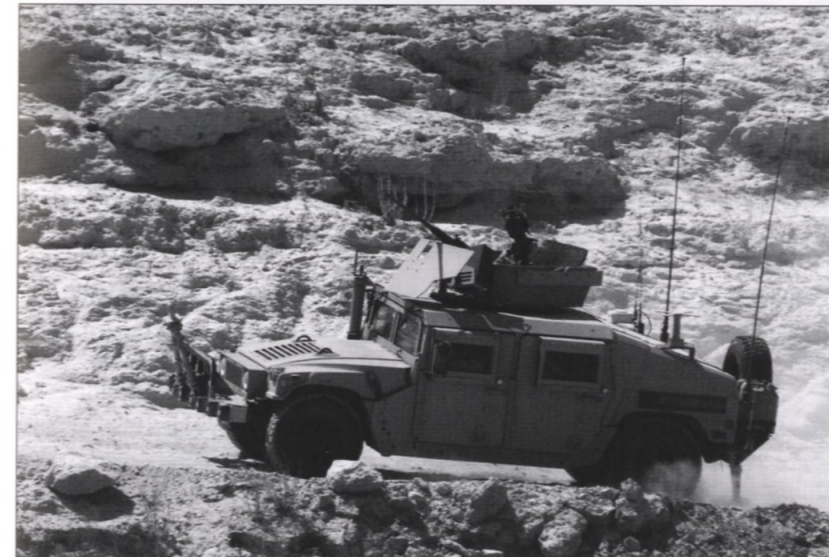
A US Army Special Forces HMMWV in Iraq, equipped with bullbars, an ASK turret for the top gunner, electronic counter-measures against Improvised Explosive Devices, and a SATCOM suite. (Courtesy CJSOFT AP PAO, photo Mass Comm Spec 2nd Class Eli J. Medellin)
