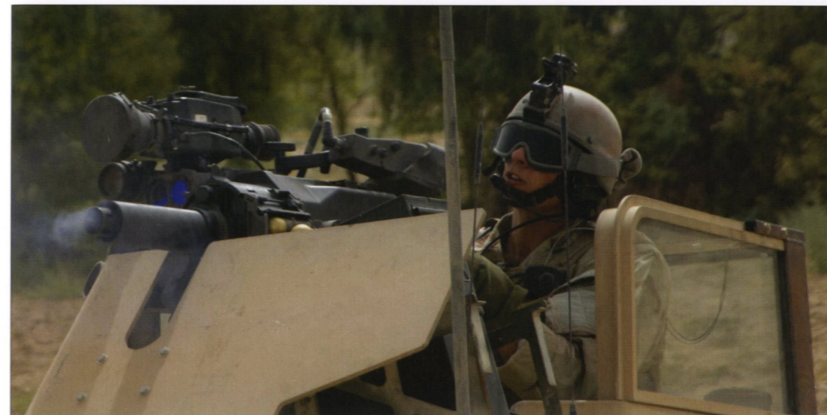
Details of the 40mm Mk47 Mod 0 Stryker automatic grenade-launcher, being test-fired from a GMV turret. Beyond the AGL is an LRAS surveillance system. (Courtesy US Navy; photo Mass Comm Spec 2nd Class Christopher Perez)
