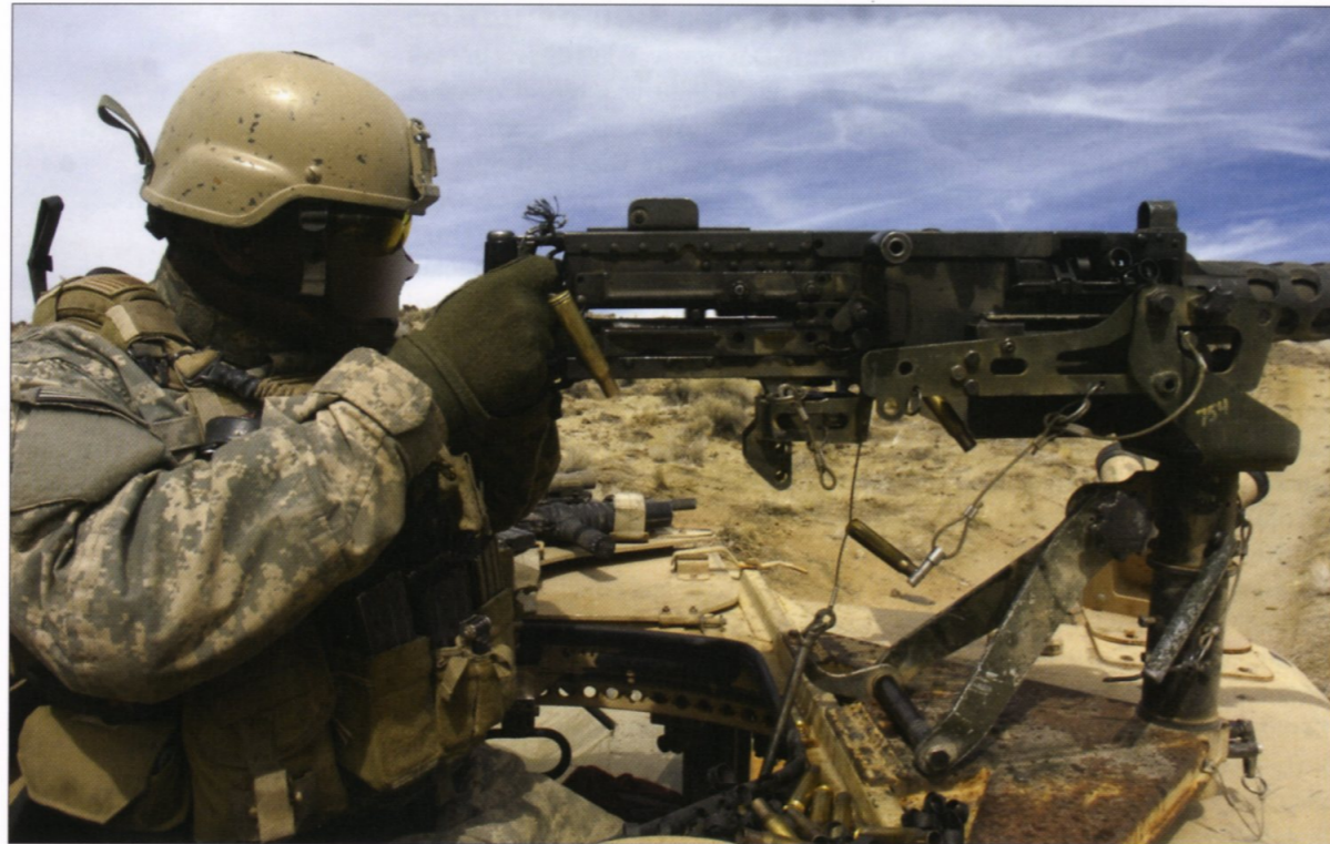
The turret gunner in a US Army Special Forces Ground Mobility Vehicle (GMV) opens fire with his .50cal M2 heavy machine gun – note the empty cases falling. No other World War II-vintage weapon in the world is still in as widespread and satisfactory use as the apparently irreplaceable ‘big fifty’. (Courtesy USSOCOM)
