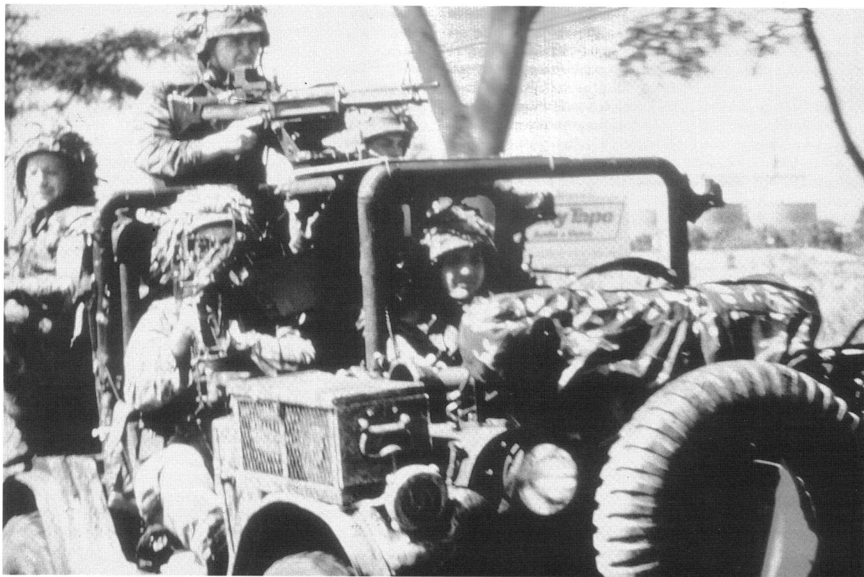
Rangers aboard a specially modified 'gun jeep' 1/4-ton M151A2 utility truck fitted with two M60 machine guns, equipment boxes, and roll bars. (DoD)
