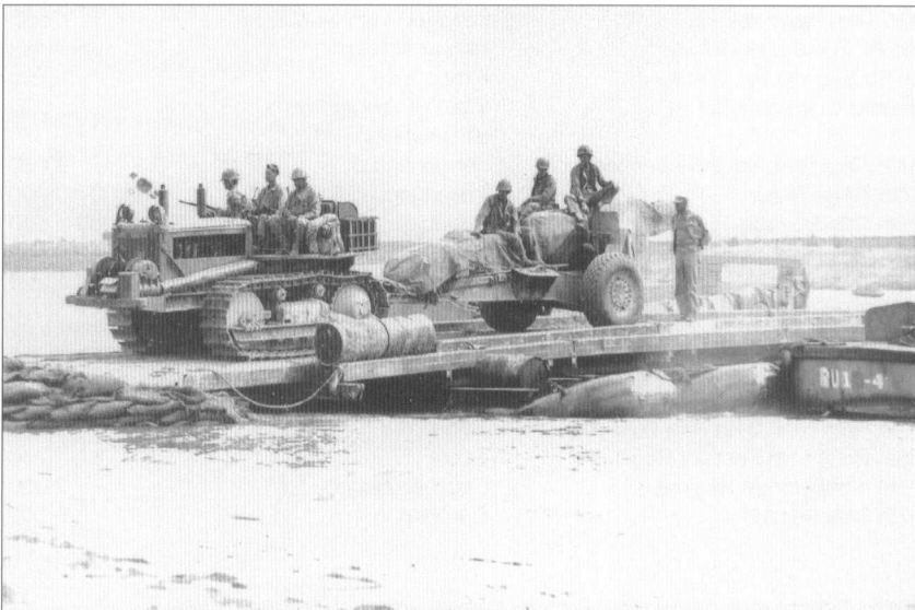
Here a marine 155mm M1A1 howitzer is towed by a dozer-tractor off a pontoon raft. Both marine and army divisions had one "155" battalion, and two battalions were assigned to X Corps, one being self-propelled. (USMC)
