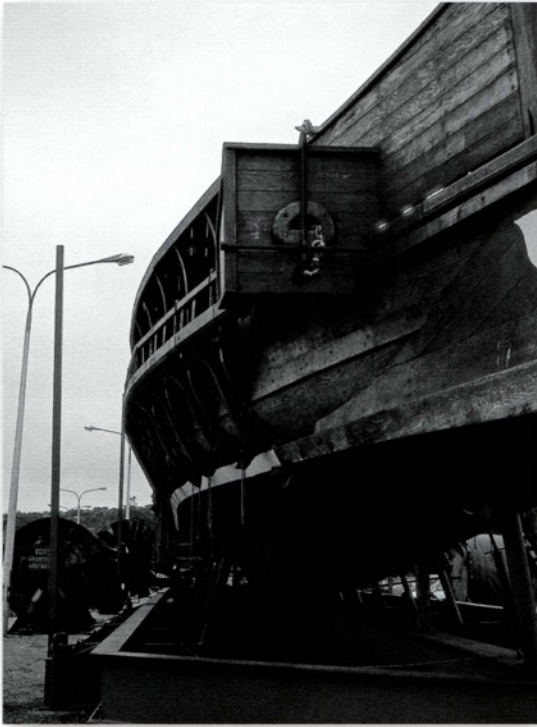
The bow of Olympias showing one of the box-like epôtides or cat-heads, which protect the outriggers. This was the structure the Syracusans reinforced with stay-beams, thereby allowing their triremes to ram the Athenians head on, bow to bow. (Fields-Carré Collection)
