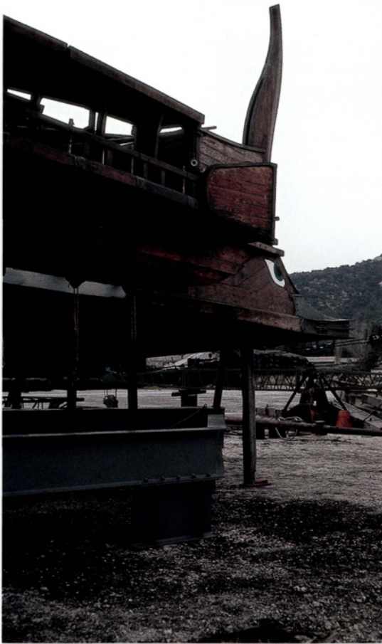
The ram was designed to cause maximum waterline damage without penetrating the hull too far and making it difficult for the attacking vessel to disengage. In Olympias , the full-scale replica of Morrison and Coates, the bronze sheath weighs some 200kg. (Fields-Carré Collection)
