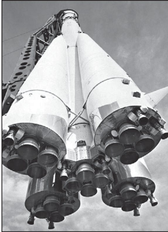
Rocket engines of the Soviet launch vehicle that was used to place manned Vostok spacecraft into orbit. Based on the R-7 intercontinental ballistic missile, the launcher had four strap-on liquid-propellant boosters surrounding the liquid-propellant core rocket. Novosti Press Agency
