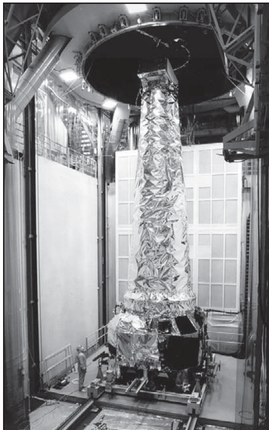
NASA's Chandra X-ray Observatory being prepared for testing in a large thermal/vacuum chamber. NASA/CXC/SAO
