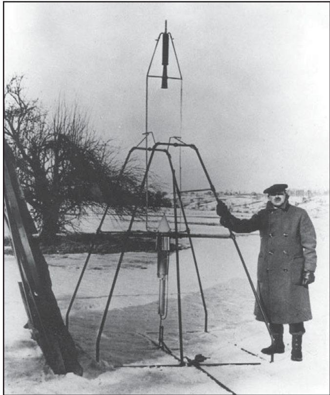
Robert H. Goddard and a liquid oxygen-gasoline rocket in its frame; the rocket was first fired on March 16, 1926, at Auburn, Mass. NASA
