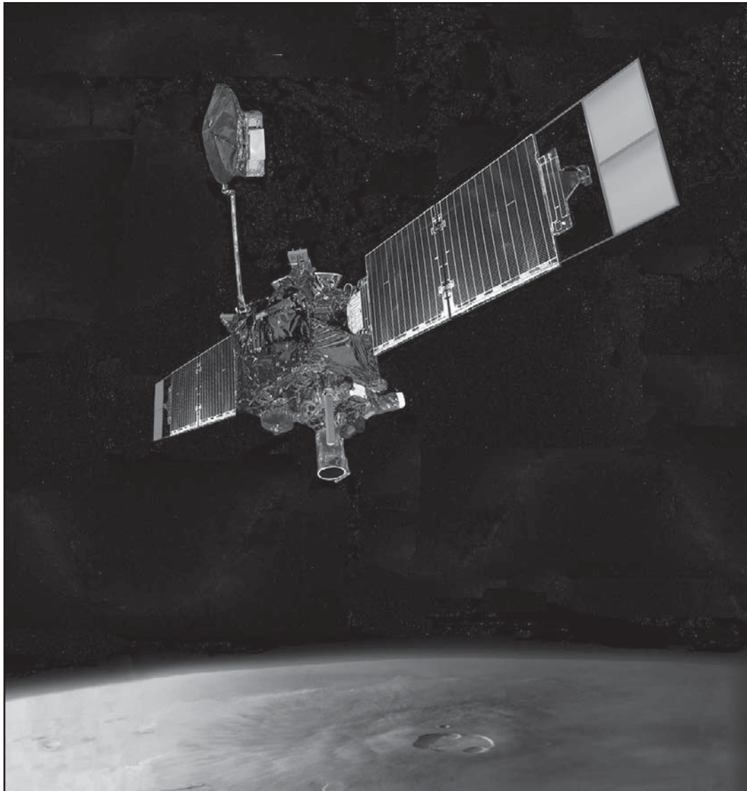
Mars Global Surveyor in orbit over the Martian volcano Olympus Mons, in an artist's conception. The spacecraft's two long solar-panel wings supply its electrical power. Tipped with drag-flap extensions, the wings also provide most of the surface area used for aerobraking the craft into its circular mapping orbit around Mars. Other prominent features are the orbiter's Earth-directed high-gain dish antenna (at top) and its Mars-facing suite of instruments, which includes a high-resolution camera and a laser altimeter. NASA/JPL/Illustration by Corby Waste
