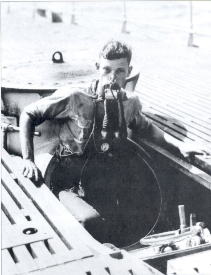
A crewman demonstrates the proper method of wearing the Momsen Lung as he moves from the aft escape trunk in this prewar photograph. (US Navy Photograph)
