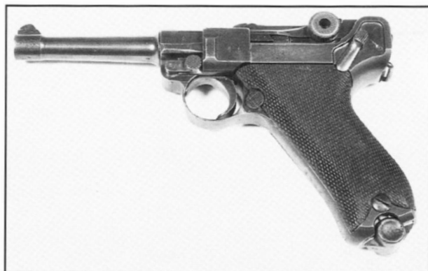
The German Army's standard service pistol was the Pistole '08, better known by the name of its inventor, the Luger. With an 8-round magazine and one in the breech, the Luger had a clear edge
