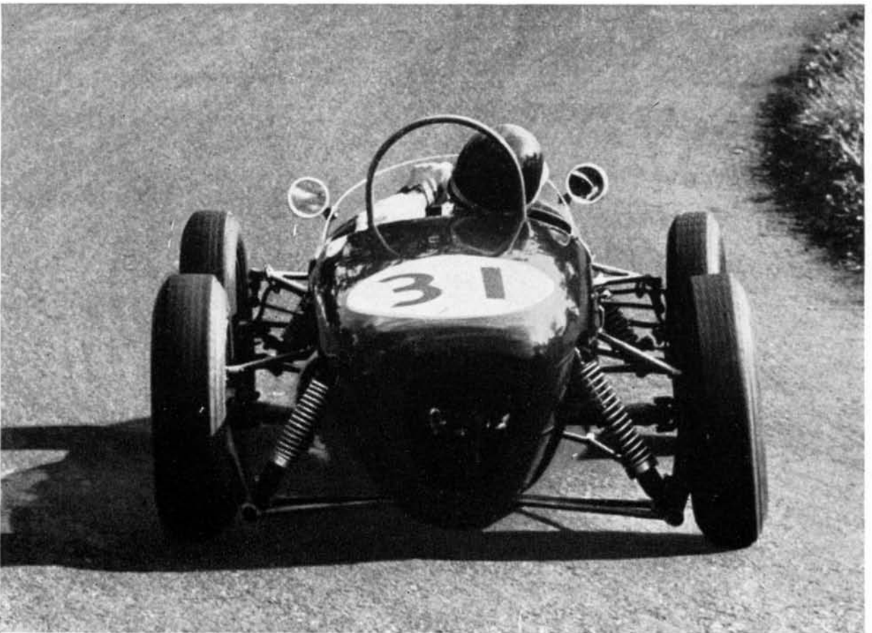
29, 30 Brabham's Formula I Cooper at Oporto (above) and Clark's Formula Junior Lotus at Oulton Park, show how the more advanced types of suspension keep the outside wheels almost upright during cornering. The camber of the lightly loaded inside wheels is far less important—as is the fact that Brabham's inside front wheel is clear of the road
