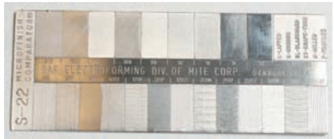
Figure C-33 Visual surface roughness comparator gage.
