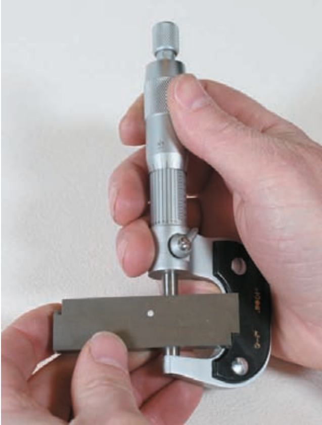
Figure C-253 Measuring the adjustable parallel with an outside micrometer.
