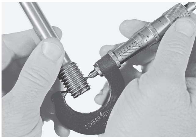
Figure C-100 Screw thread comparison micrometer measuring a screw thread.
