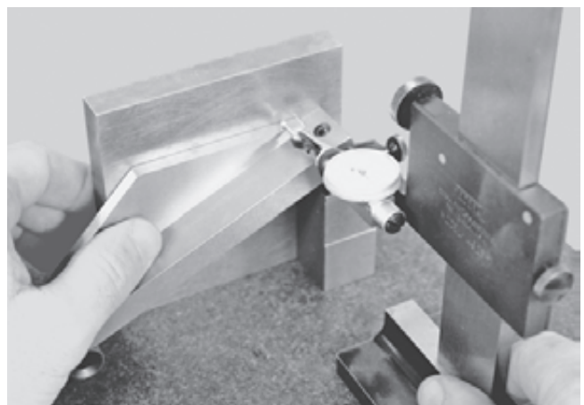
Figure C-255 Placing the gage block stack under the sine bar.
