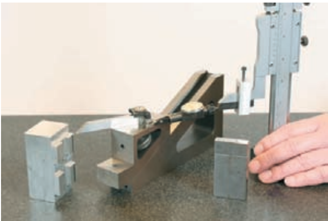
Figure C-173 Transferring the measurement to the planer gage.
