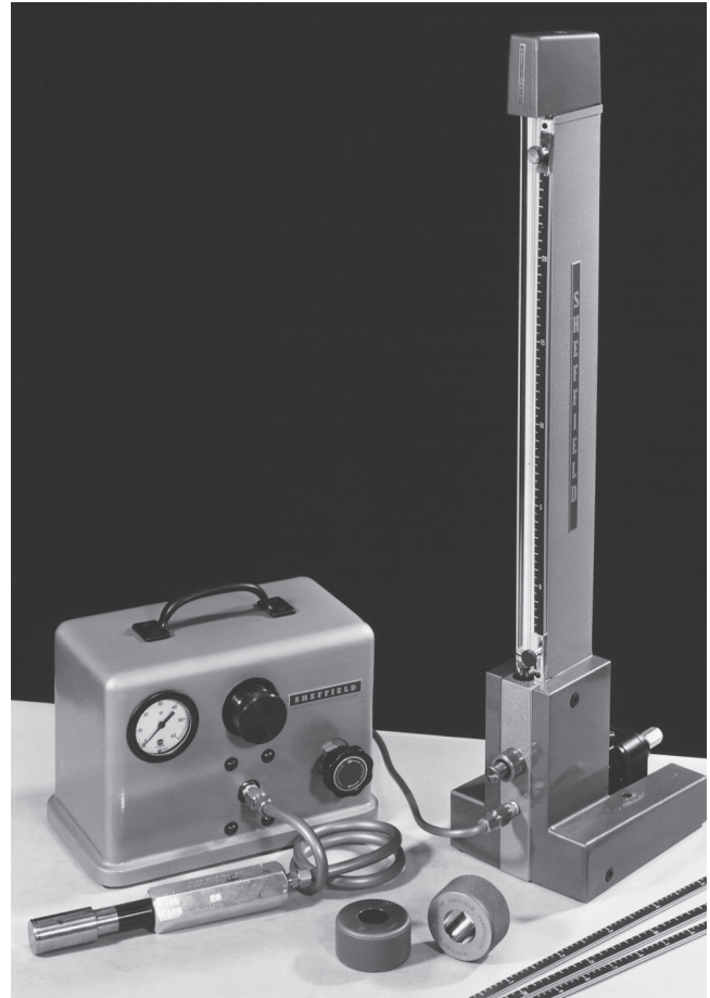
Figure C-16 Column or flow-type air gage (Besly Cutting Tools, Inc.).
