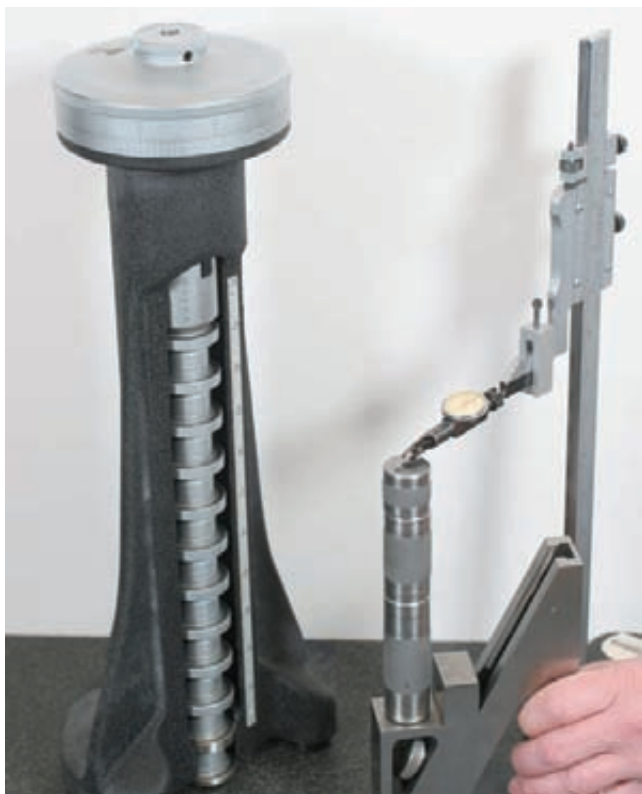
Figure C-201 Transferring the measurement to the planer gage.
