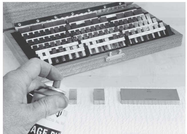
Figure C-215 Applying gage block cleaner.
