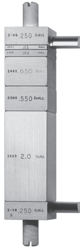
Figure C-232 Gage block stack with accessory gage pins (Courtesy of DoALL Company).
