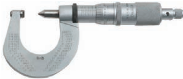
Figure C-99 Screw thread comparison micrometer.
