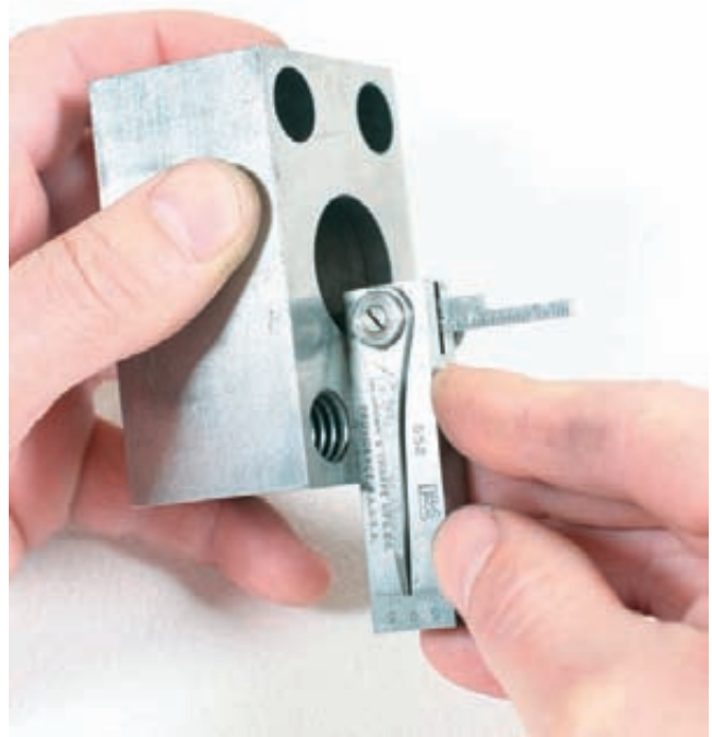
Figure C-183 Using the diemaker's square to check die clearance angle.
