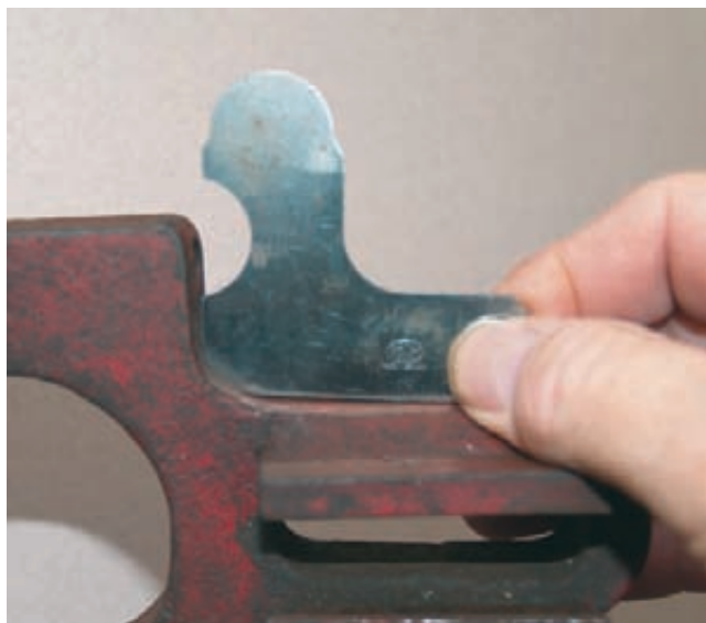
Figure C-170 Using a feeler or thickness gage (Courtesy of The L.S. Starrett Co.).
