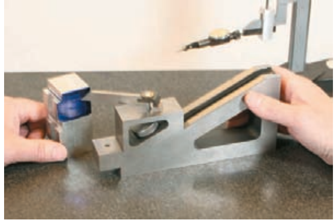
Figure C-174 Using the planer gage in layout.
