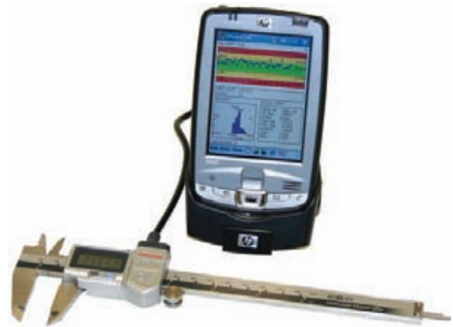
Figure C-263 The digital caliper is an example of SPC equipment for dimensional measurement of machined parts. The attached microprocessor records, graphs, and prints part dimensions and generates appropriate statistical data (Mitutoyo America Corp.).
