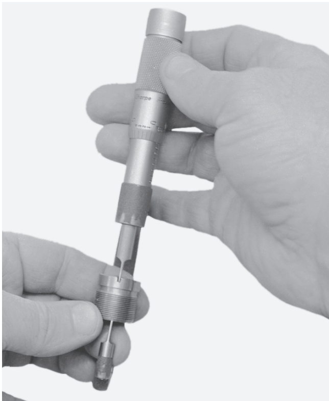
Figure C-96 Blade micrometer measuring a groove.
