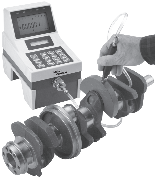
Figure C-14 Pressure-type air snap gage (Courtesy Mahr Federal Inc.).
