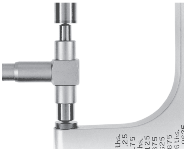
Figure C-162 Checking the telescoping gage with an outside micrometer.
