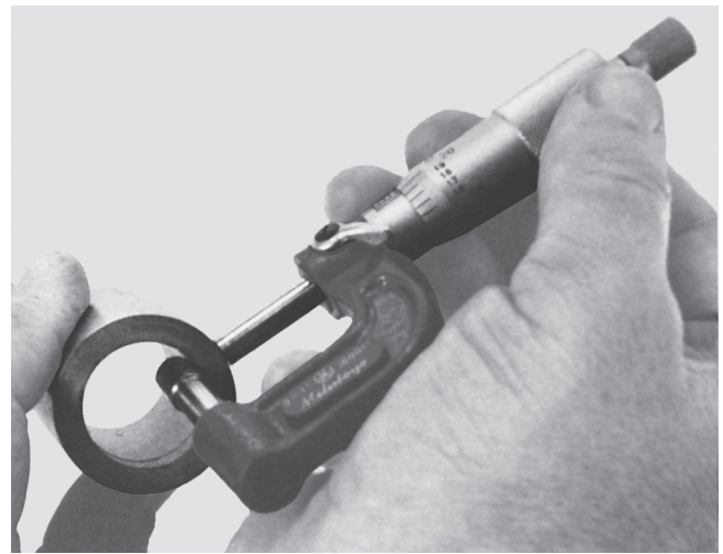
Figure C-114 Tubing micrometer measuring a tube wall.
