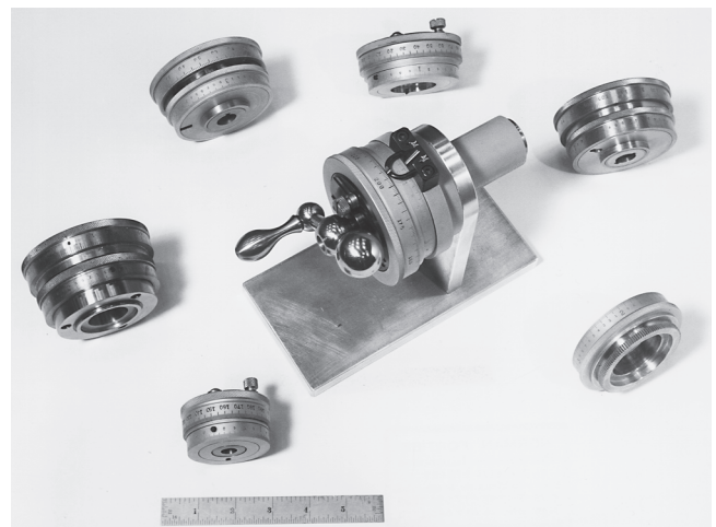
Figure C-47 Inch/metric conversion dials for machine tools (Sipco Machine Company).
