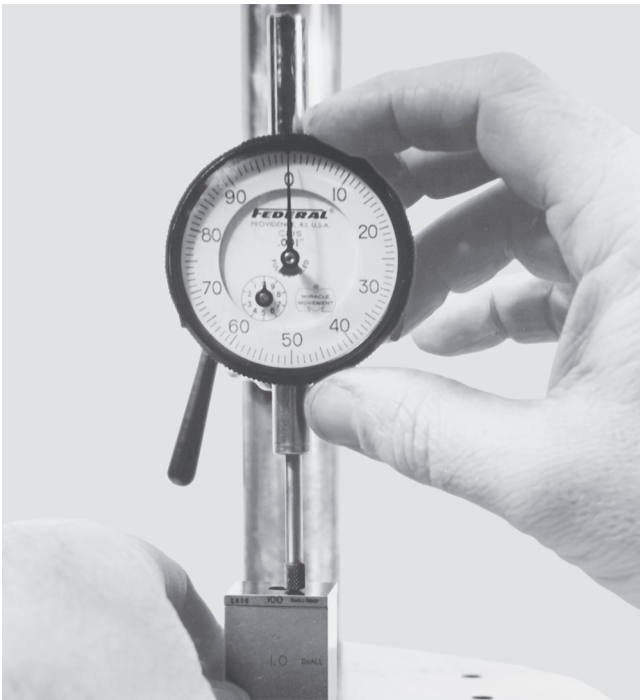
Figure C-205 Setting the dial indicator to zero using gage blocks.
