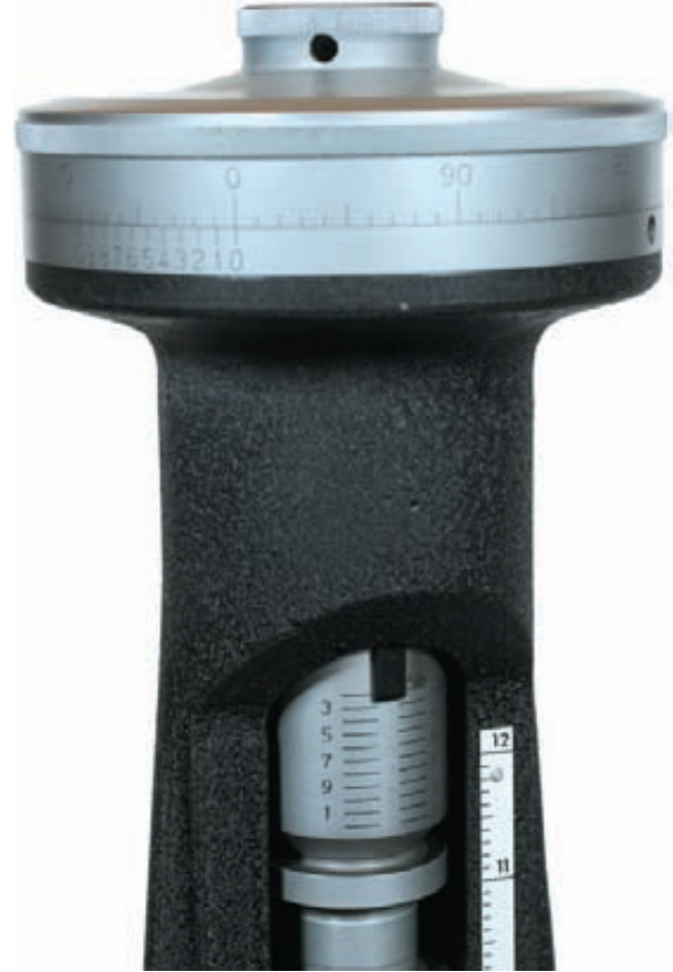
Figure C-199 Reading the precision height gage.
