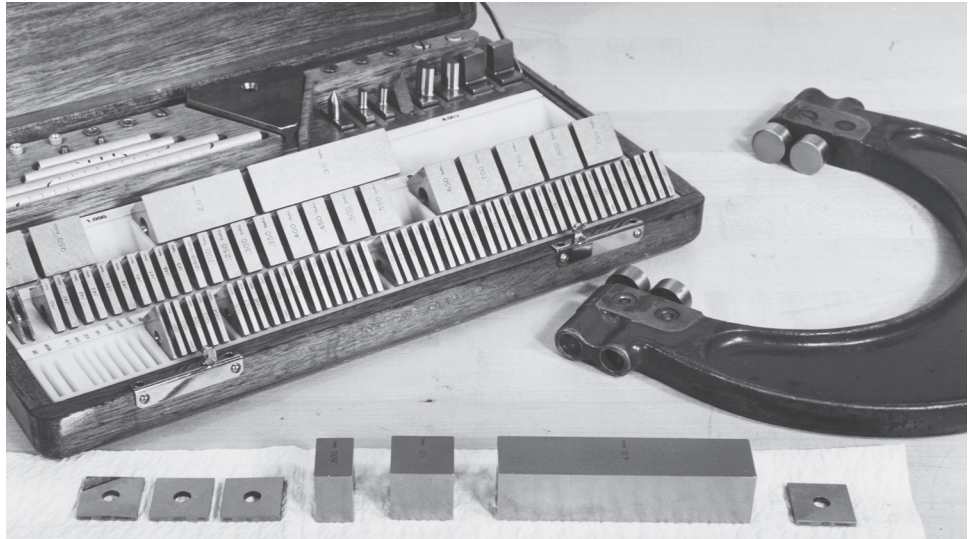
Figure C-227 Gage and wear blocks for setting a snap gage.
