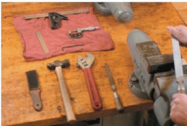
Figure C-124 Micrometers should be kept on a clean shop towel when used on the bench.
