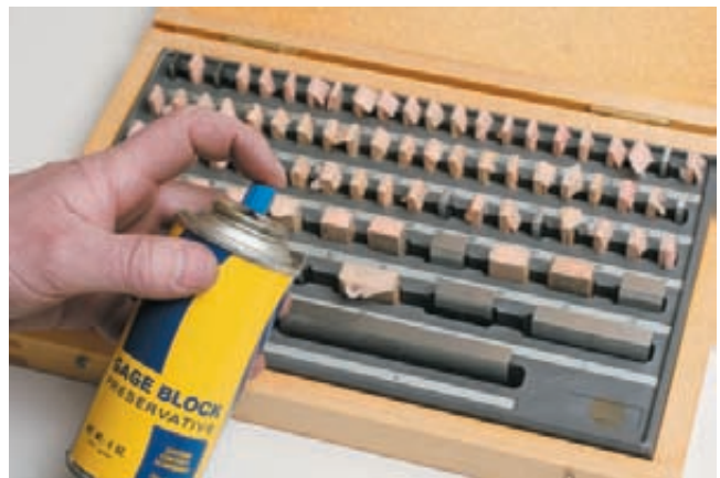
Figure C-226 Applying gage block preservative.
