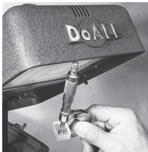
Figure C-42 Using optical flats to check micrometer measuring faces (Courtesy of DoALL Company).
