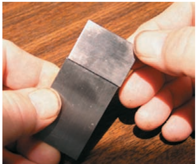
Figure C-218 Wrung gage blocks in line.
