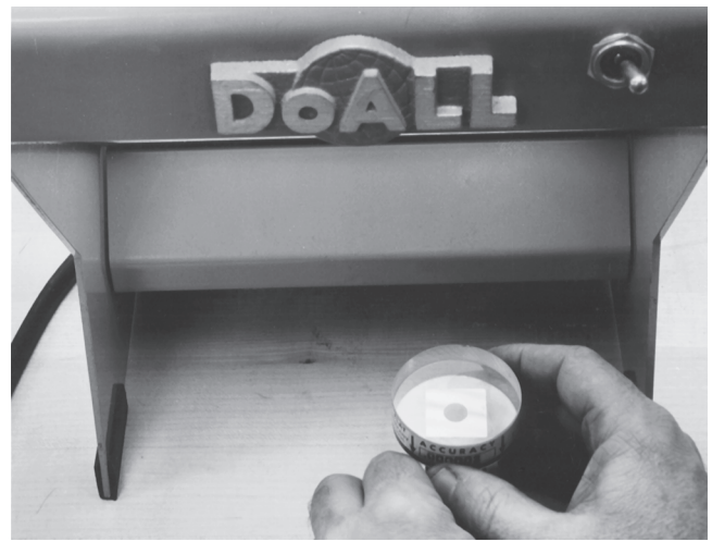
Figure C-221 Inspecting a gage block under monochromatic light.
