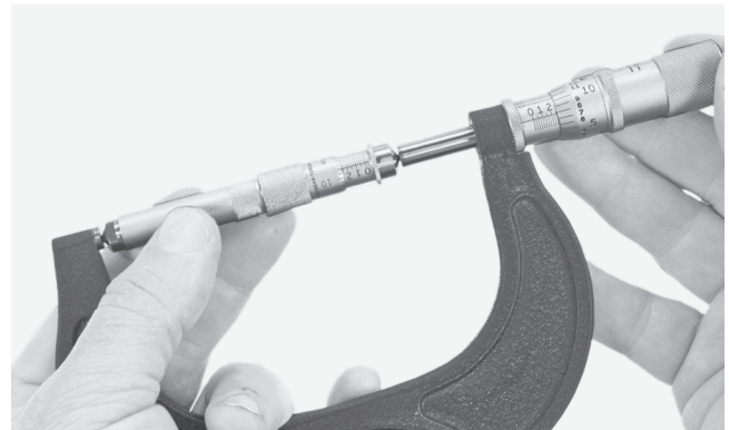
Figure C-140 Checking the inside micrometer with an outside micrometer.
