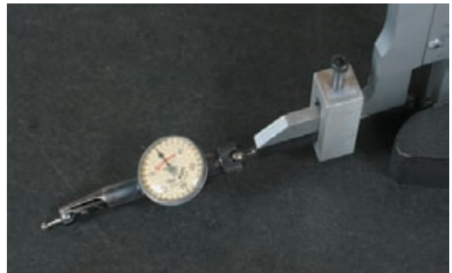
Figure C-196 Setting the dial test indicator to zero on the reference surface.
