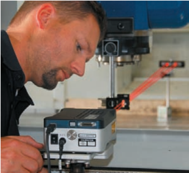
Figure C-45 Laser interferometer being used for straightness determination (Courtesy of Renishaw).
