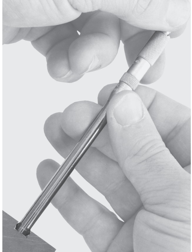
Figure C-166 Using the twin ball small hole gage.
