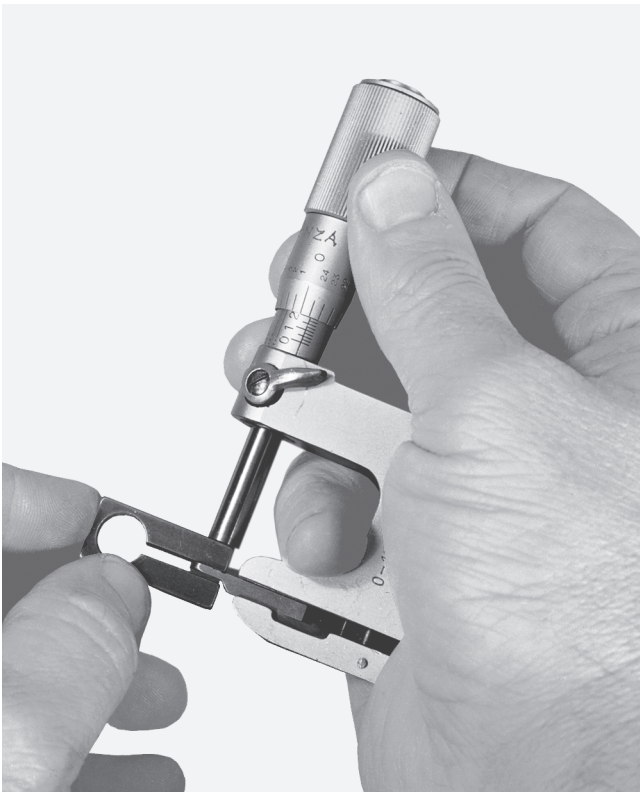
Figure C-108 Interchangeable anvil micrometer with flat anvil.
