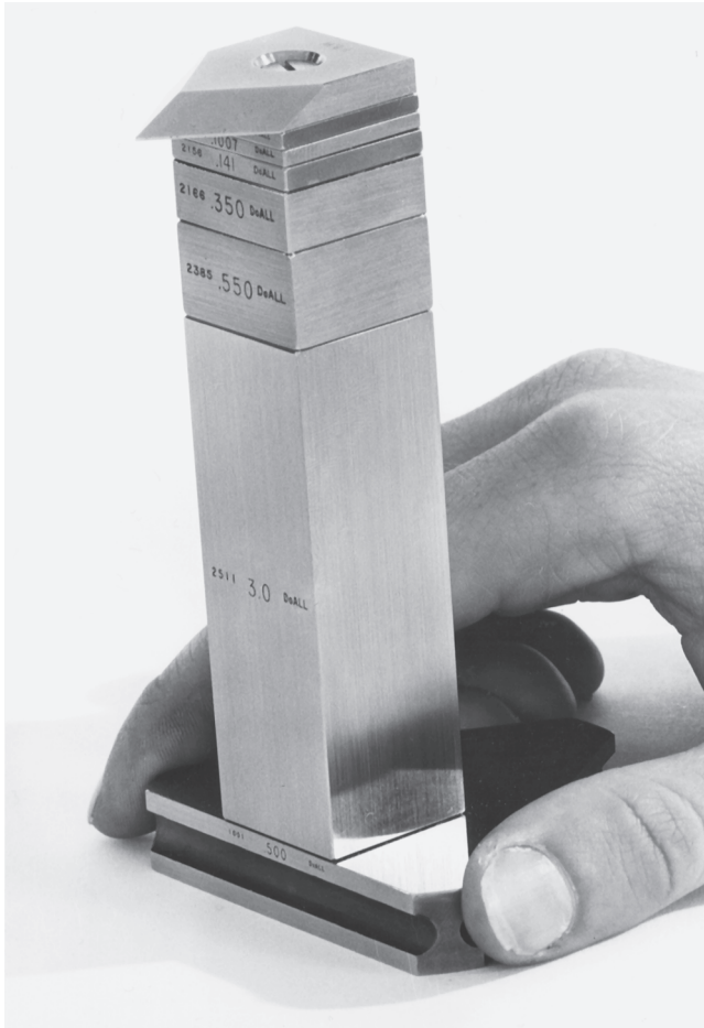
Figure C-231 Precision height gage assembled from gage blocks (Courtesy of DoALL Company).
