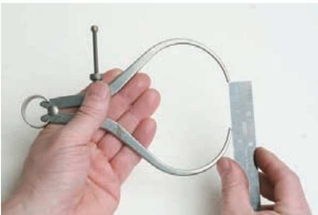
Figure C-156 Comparing the spring caliper with a steel rule.
