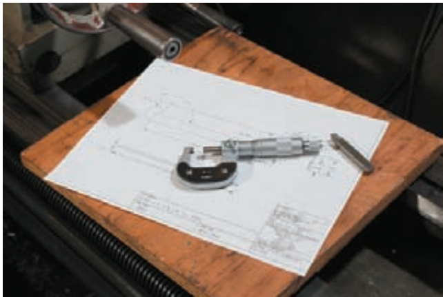
Figure C-123 Micrometers should always be kept on a tool board when used near a machine tool.
