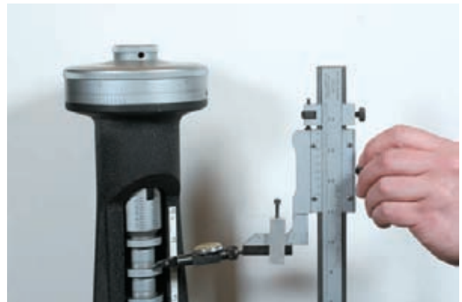
Figure C-200 Setting the dial test indicator to the precision height gage.
