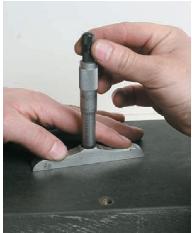
Figure C-145 Checking a depth micrometer for zero adjustment using the surface plate as a reference surface.
