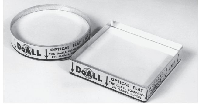
Figure C-220 Round and square optical flats (Courtesy of DoALL Company).
