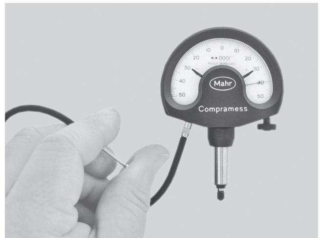
Figure C-207 Dial indicator comparator with cable lift.
