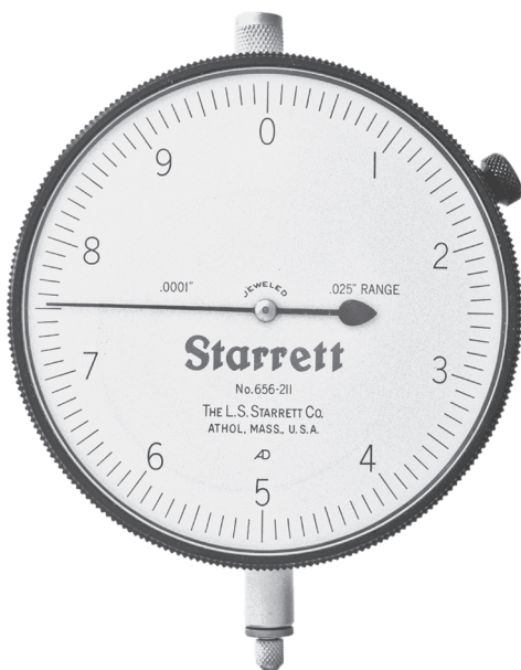
Figure C-187 Dial indicator with .025-in. range and .0001-in. discrimination.
