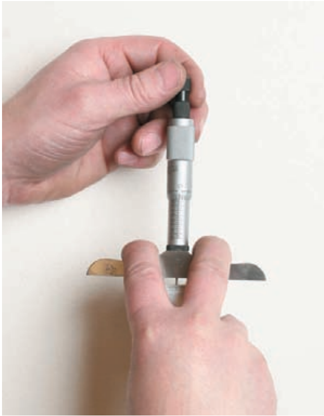
Figure C-143 Proper way to hold the depth micrometer.
