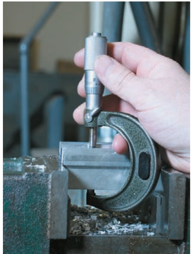
Figure C-131 Read a micrometer while it is still in contact with the workpiece.
