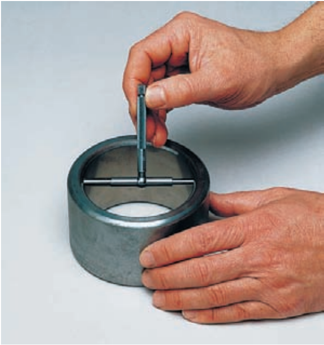
Figure C-159 Inserting the telescoping gage into the bore (Courtesy of The L.S. Starrett Co.).
