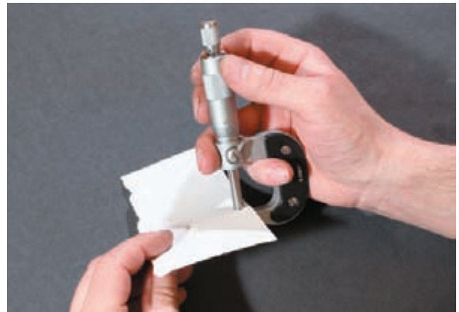
Figure C-125 Cleaning the measuring faces.
