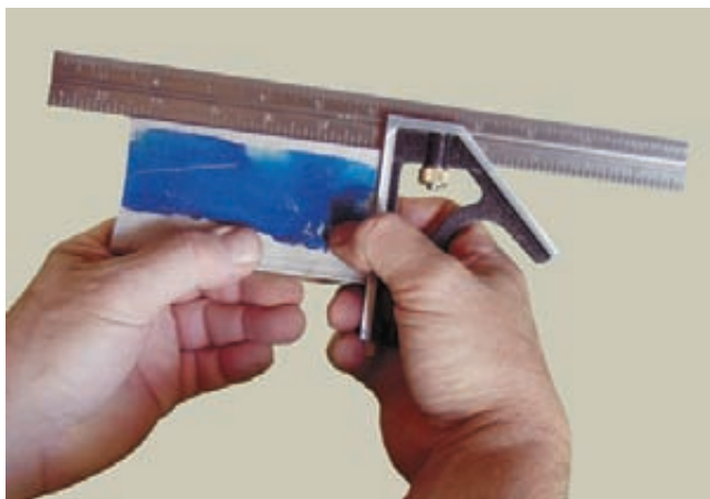
Figure C-177 Using the combination square.
