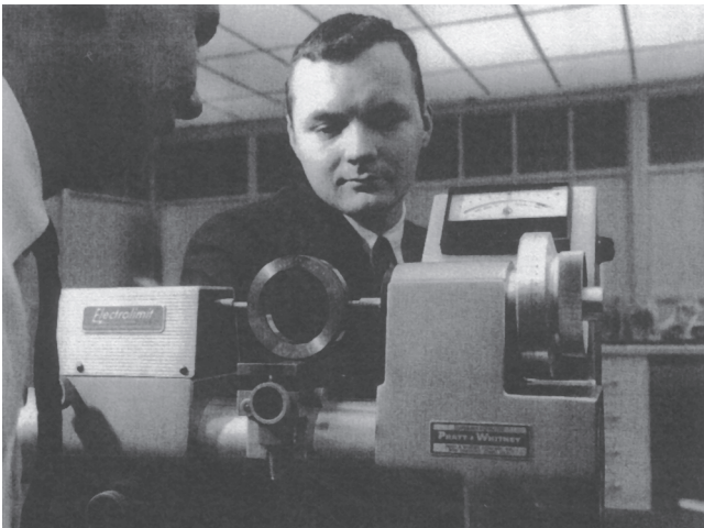
Figure C-31 Using a micrometer to measure a workpiece.
