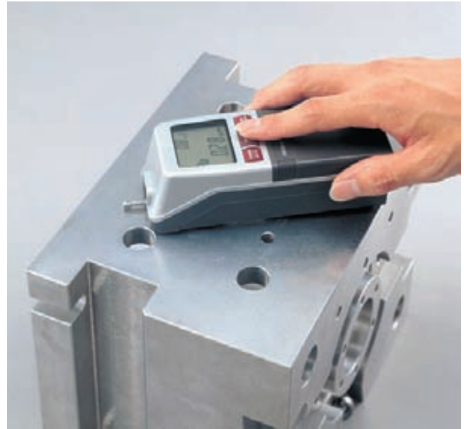
Figure C-36 Surface roughness instrument used to check a machined surface (Mitutoyo America Corp.).
