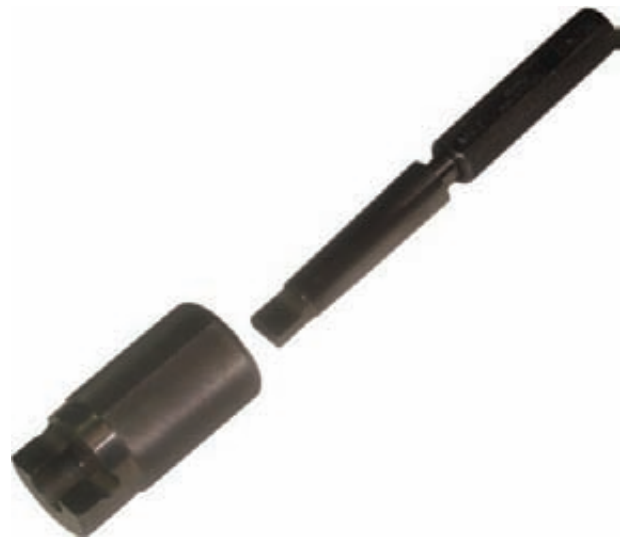
Figure C-9 Taper plug and taper ring gage (Courtesy Prof. Frank Mueck, Cambrian College of Applied Arts and Technology Tool and Die Machining).
