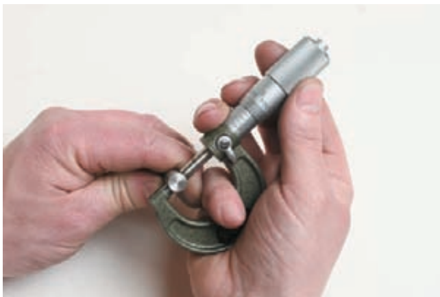
Figure C-130 Proper way to hold a micrometer.
