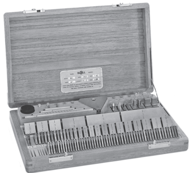
Figure C-214 Gage block set with accessories (Courtesy of DoALL Company).
