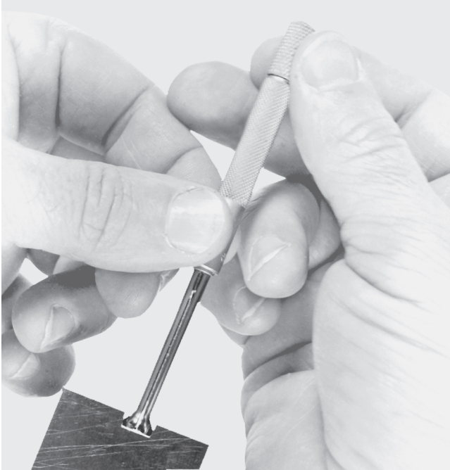
Figure C-164 Insert the small hole gage in the slot to be measured.
