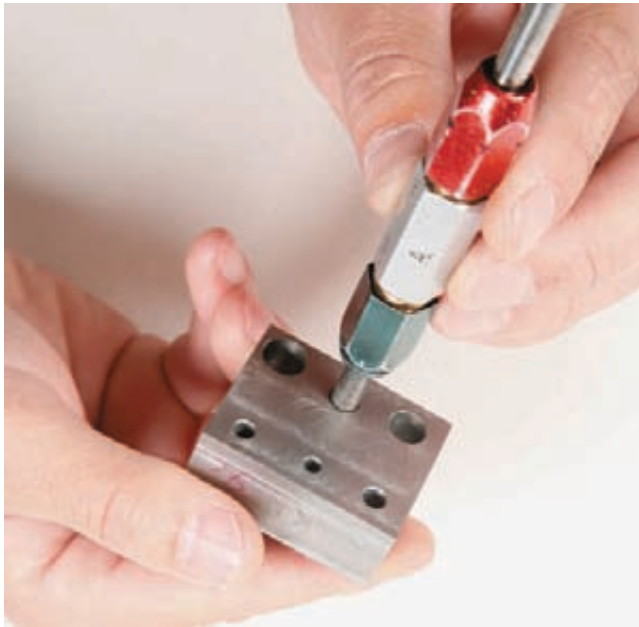
Figure C-10 Using the cylindrical plug gage (Courtesy Terra Community College).
