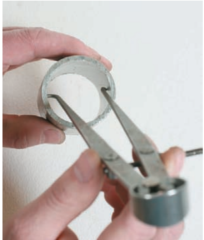
Figure C-157 Using an inside spring caliper.
