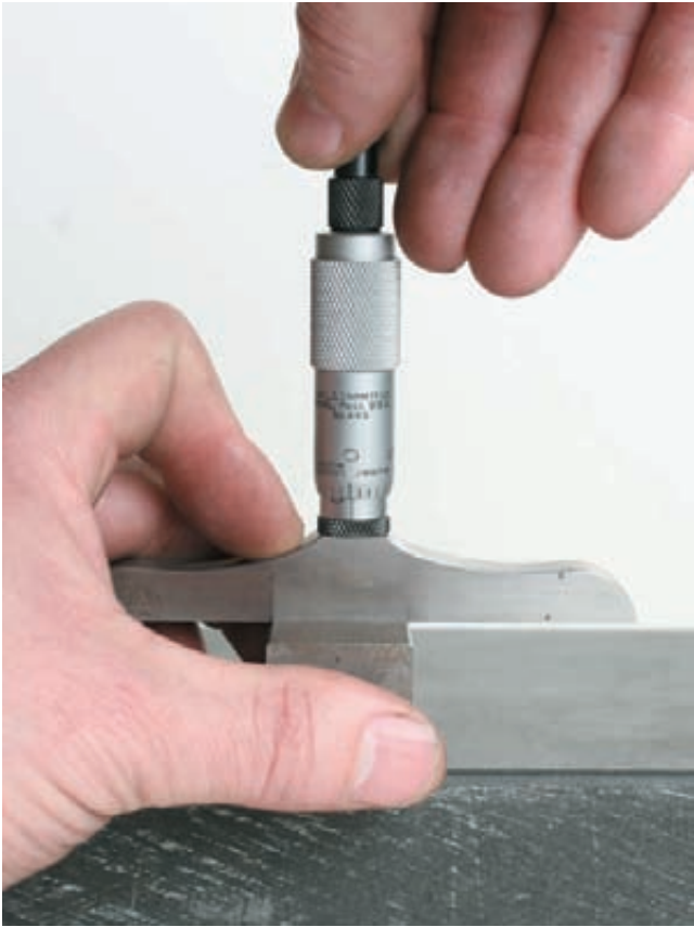
Figure C-146 Checking the depth micrometer calibration at the 1.000-in. position in the 0- to 1-in. rod, and a 1-in. square or Hoke gage block.
