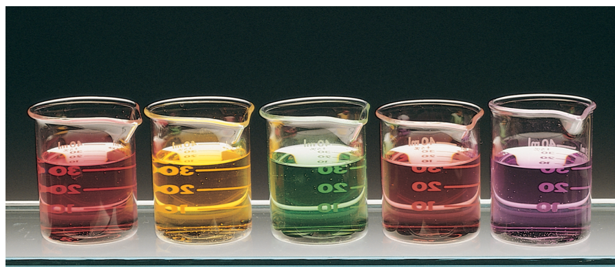
FIG. 21.24 Colors of complex ions depend on the nature of the ligands. Each of these brightly colored solutions contains a complex ion of \text{Co}^{3+} . The variety of colors arises because of the different ligands (molecules or anions) that are bonded to the cobalt ion in the complexes. (Michael Watson.)
