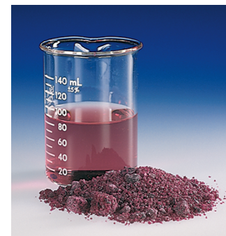
FIG. 21.14 Color of the cobalt(II) ion in hexahydrate salts. The ion [\text{Co}(\text{H}_2\text{O})_6]^{2+} is pink and gives its color both to crystals and to an aqueous solution of \text{CoCl}_2 \cdot 6\text{H}_2\text{O} . (Michael Watson.)
