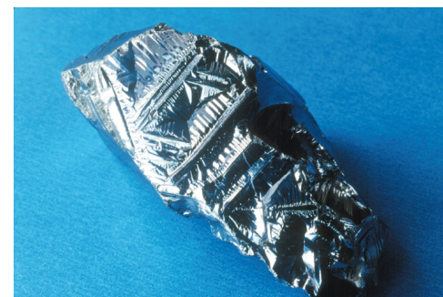
A sample of crystalline elemental silicon exhibits a metallic sheen. (Jeff J. Daby/ Fundamental Photographs .)
