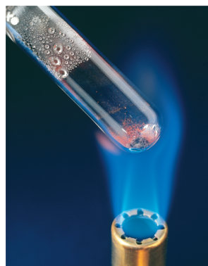
FIG. 21.9 Thermal decomposition of mercury(II) oxide. Heated to a temperature of only 400 °C, HgO turns black and releases oxygen. Drops of mercury metal begin to collect on the walls of the test tube as mercury vapor condenses on the cooler parts of the tube. (Richard Megna/Fundamental Photographs.)
