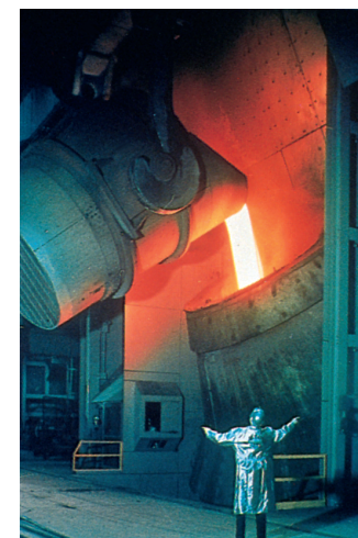
A molten iron charge is added to a basic oxygen furnace. (James Mejuto Photography.)
