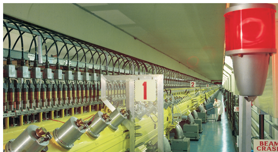
FIG. 20.10 Linear accelerator. In this linear accelerator at Brookhaven National Laboratory on Long Island, New York, protons can be accelerated to just under the speed of light and given up to 33 GeV of energy before they strike their target. (1 GeV = 10^9 eV.) (Courtesy Brookhaven National Laboratory.)
