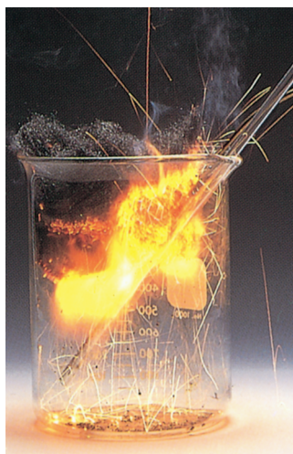
FIG. 13.4 Effect of concentration on rate. Steel wool, after being heated to redness in a flame, burns spectacularly when dropped into pure oxygen. (OPC, Inc.)
