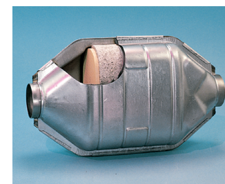
FIG. 13.19 A modern catalytic converter of the type used in about 80% of new cars. Part of the converter has been cut away to reveal the porous ceramic material that serves as the support for the catalyst. (Courtesy AC Spark Plug)
