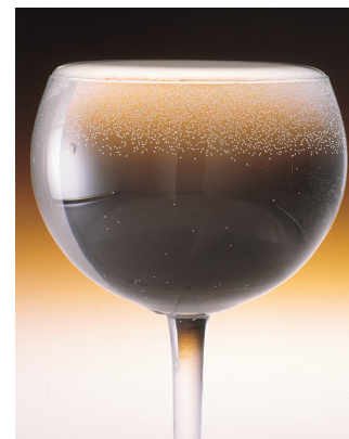
FIG. 11.14 Surface tension in a liquid. Surface tension allows a glass to be filled with water above the rim. (Michael Watson.)
