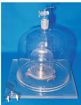
FIG. 1.14 The international standard kilogram. This standard for mass in the SI is made of a platinum–iridium alloy and is kept at the International Bureau of Weights and Measures in France. Other nations such as the United States maintain their own standard masses that have been carefully calibrated against this international standard. (Courtesy Bureau International des Poids et Mesures.)
