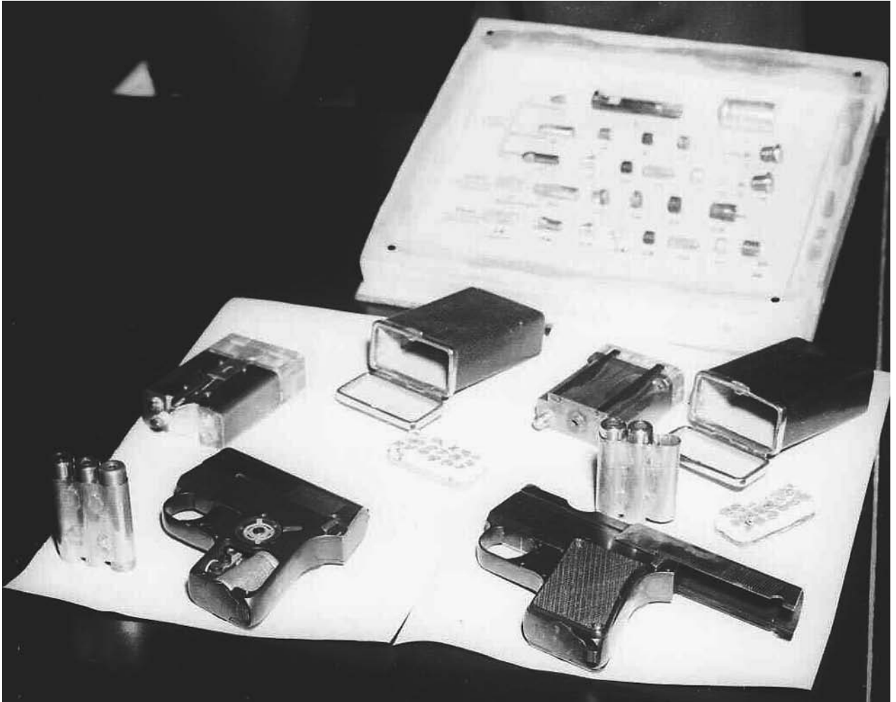
Concealed weapons that fell into western hands through the defection of Russian Intelligence Captain Nikolai E. Khokhlov in 1954 included cases of cigarettes that fired hollowpoint bullets and miniature pistols that fired while making a sound less than the snap of a finger. AP/WIDE WORLD PHOTOS.
