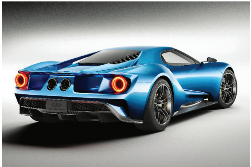
Ford's GT supercar uses carbon fiber composites on its body panels and inner rear deck.
