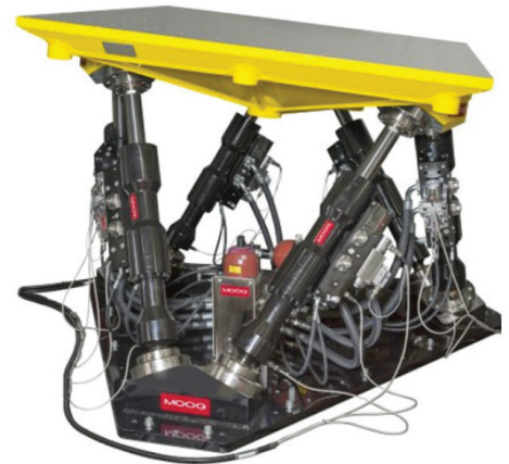
Moog hydraulic simulation table ordered by Thule.
