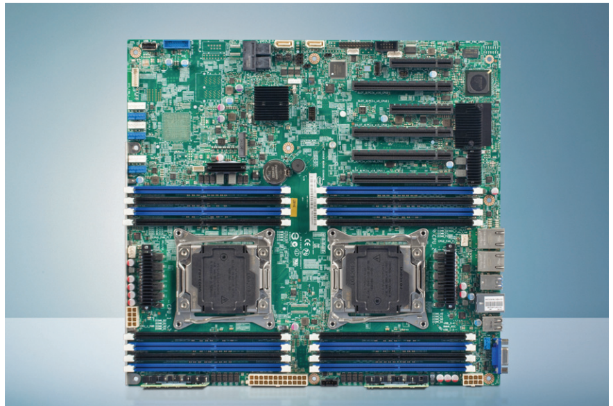
The new C6670 industrial server from Beckhoff offers options for two Intel Xeon processors each with 6, 12, or 18 cores on one motherboard.
